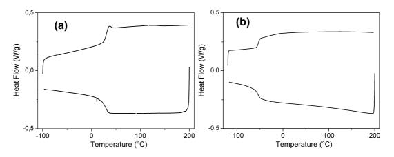
Figure IV.30. DSC at 10°C/min (exo down) of (a) DAT-PPO-460-DAT 2b and (b) DAT-PPO-2200-DAT 2a.
