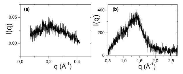
Figure IV.32. (a) SAXS and (b) WAXS spectra, of DAT-PPO-2200-DAT 2a at room temperature.<sup>33</sup>
