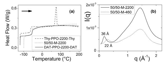
**Figure IV.35.** (a) DSC at 10°C/min (exo down) of DAT-PPO-2200-DAT <u>2a</u>, 50/50-M-2200 <u>4a</u>, Thy-PPO-2200-Thy <u>3a</u>; (b) X-ray scattering at 25°C of 50/50-M-X <u>4a-b</u>.
