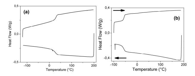
Figure IV.36. DSC at 10°C/min (exo down) of (a) 50/50-M-460 4b and (b) 50/50-M-2200 4a.
