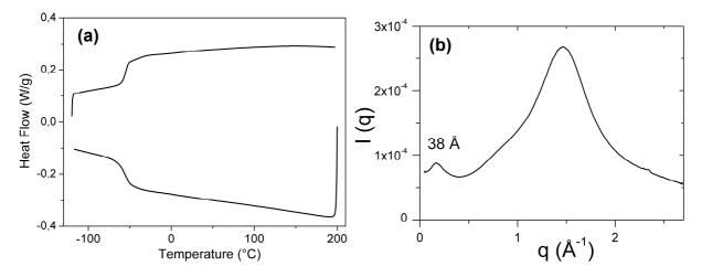
Figure IV.40. (a) DSC at 10°C/min (exo down) and (b) X-ray scattering spectra at 25°C, of 25/75-M-2200 5a.
