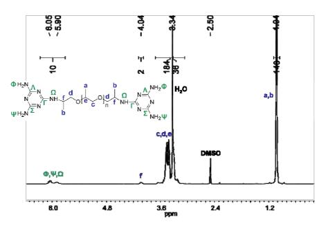
Figure 2. <sup>1</sup>H NMR in DMSO-d<sub>6</sub> of DAT-PPO-2200-DAT <u>2a</u>.
