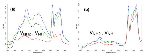
Figure IV.45. FT-IR of stickers' bonds involved in hydrogen bonding at 30°C (in blue), 100°C (in green) and 180°C (in red) of (a) DAT-PPO-460-DAT <u>2b</u> and (b) DAT-PPO-2200-DAT <u>2a</u>.
