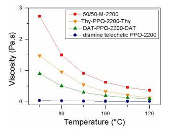
Figure IV.43. Viscosity as a function of temperature for diamine telechelic NH<sub>2</sub>-PPO-2200-NH<sub>2</sub> <u>1a</u>, DAT-PPO-2200-DAT <u>2a</u>, Thy-PPO-2200-Thy <u>3a</u>, and 50/50-M-2200 <u>4a</u>.
