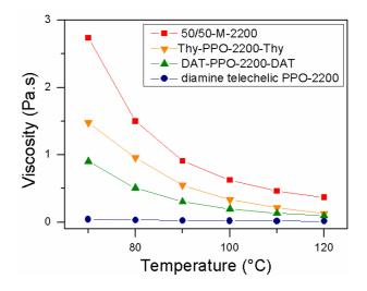
Figure V.4. Viscosity as a function of temperature for diamine telechelic NH<sub>2</sub>-PPO-2200-NH<sub>2</sub> <u>1a</u>, DAT-PPO-2200-DAT <u>2a</u>, Thy-PPO-2200-Thy <u>3a</u>, and 50/50-M-2200 <u>4a</u>.
