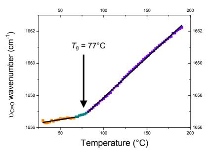
**Figure V.1.**  $T_{g}$  determination of Thy-PPO-250-Thy <u>**3c**</u> by temperature-dependant FT-IR in ATR mode (this sample contained impurities so  $T_{g}$  was lower than for the more pure Thy-PPO-250-Thy <u>**3c**</u> discussed in the following pages).
