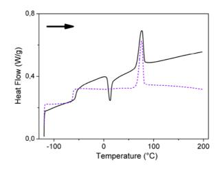
Figure V.3. DSC on heating of Thy-PPO-2200-Thy <u>3a</u> at 10°C/min (exo down) after cooling at: (a) 10°C/min (dot-line) and (b) 60°C/min (full line).
