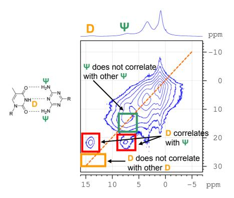
**Figure IV.39.** 2D bulk <sup>1</sup>H NMR at 25°C (correlation simple quanta <sup>1</sup>H – double quanta <sup>1</sup>H) of 50/50-PPO-460 <u>**4b**</u>. On the horiontal axis and on the spectra above the card is the simple quanta <sup>1</sup>H NMR (simple impulsion). On the vertical axis is the double quanta <sup>1</sup>H NMR ("BaBa" excitation of double quanta, one rotation, excitation time = 16.6  $\mu$ s). Rotation speed is 60 kHz.
