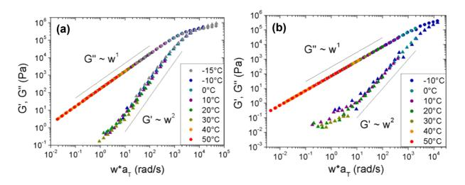
Figure IV.37. Frequency sweeps at different temperatures, shifted according to time-temperature superposition of (a) 50/50-M-2200 <u>4a</u> and (b) 25/75-M-2200 <u>5a</u>.
