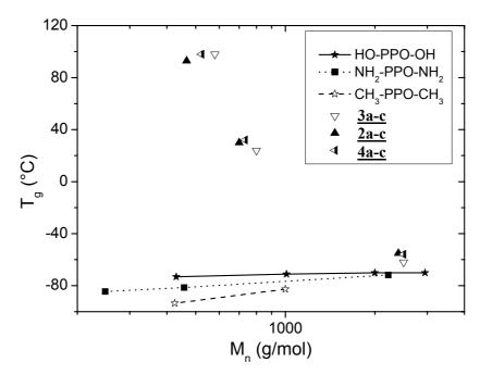
**Figure V.2.**  $T_g$  as a function of  $M_n$ , for HO-PPO-OH (from ref 8), NH<sub>2</sub>-PPO-X-NH<sub>2</sub> <u>1a-c</u>, CH<sub>3</sub>-PPO-CH<sub>3</sub> (from ref 7), Thy-PPO-X-Thy <u>3a-c</u>, DAT-PPO-X-DAT <u>2a-c</u>, and 50/50-M-X <u>4a-c</u>.
