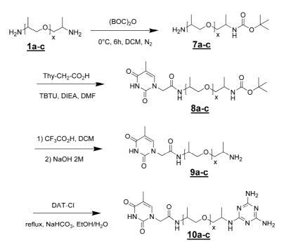
Scheme 1. Synthesis of heterotelechelic units Thy-PPO-X-DAT <u>10a-c</u> (a: X = 2200, b: X = 460, c: X = 250).
