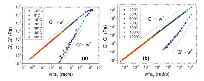
Figure IV.33. Frequency sweeps at different temperatures, shifted according to time-temperature superposition of (a) DAT-PPO-2200-DAT <u>2a</u> and (b) DAT-PPO-460-DAT <u>2b</u>.
