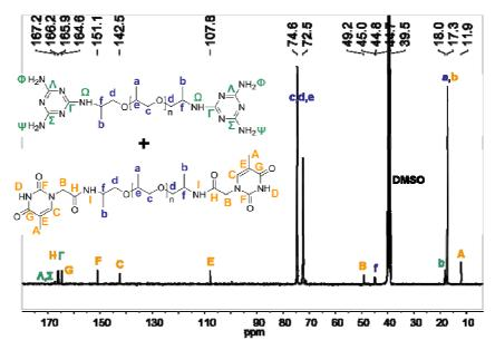
**Figure 7.** <sup>13</sup>C NMR in DMSO-d<sub>6</sub> of 50/50-M-2200 <u>4a</u>.
