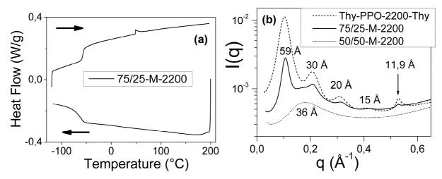
Figure IV.41. (a) DSC at 10°C/min (exo down) of 75/25-M-2200 <u>6a</u>; (b) X-ray scattering at 25°C of 75/25-M-2200 <u>6a</u>, 50/50-M-2200 <u>4a</u> and Thy-PPO-2200-Thy <u>3a</u>.
