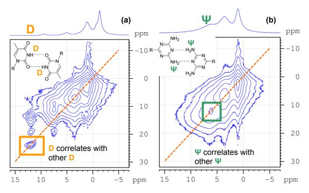
Figure IV.38. 2D bulk <sup>1</sup>H NMR at 25°C (correlation simple quanta <sup>1</sup>H – double quanta <sup>1</sup>H) of: (a) Thy-PPO-460-Thy <u>3b</u> and (b) DAT-PPO-460-DAT <u>2b</u>. Rotation speed is 60 kHz. On the horiontal axis and on the spectra above the card is the simple quanta <sup>1</sup>H NMR (simple impulsion). On the vertical axis is the double quanta <sup>1</sup>H NMR ("BaBa" excitation of double quanta, one rotation, excitation time = 16.6 μs).
