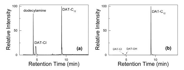
Figure 1. GC of reaction mixture: (a) after 2h, and (b) after 20h.
