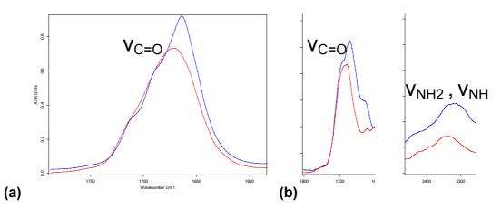
**Figure IV.44.** FT-IR of stickers' bonds involved in hydrogen bonding (a) Thy-PPO-460-Thy <u>**3b**</u> at 60°C (in blue) and 120°C (in red) and (b) 50/50-M-460 <u>**4b**</u> at 30°C (in blue) and 180°C (in red).
