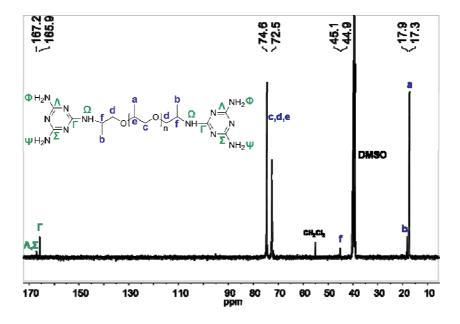
Figure 3. <sup>13</sup>C NMR in DMSO-d<sub>6</sub> of DAT-PPO-2200-DAT <u>2a</u>.
