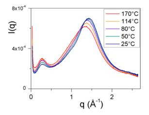
Figure IV.31. X-ray scattering spectra of DAT-PPO-460-DAT 2b at different temperatures.<sup>32</sup>
