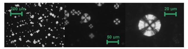
Figure IV.42. Polarized optical microscopy of 75/25-M-2200 6a.
