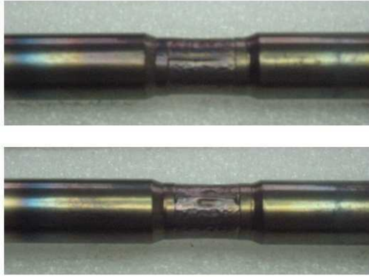
Figure 6.20: The experiment set up when interrupted at 600^{\circ}\text{C} because of the aluminium cover break, the leak mark is visible on the photo of the bottom
