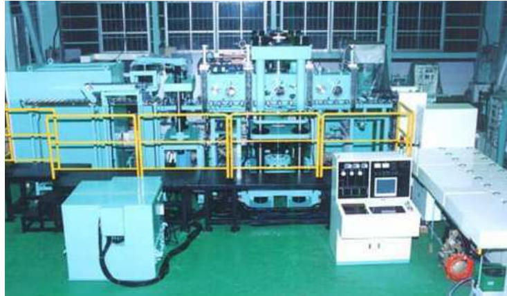
Figure 2.4: A fully automated tunnel-type sintering system developed by Fuji Electronic Industrial Co., Ltd. [1]
