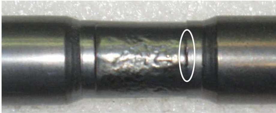
Figure 6.19: The set up when the experiment is interrupted at 680^{\circ}\text{C} , the circle shows the crack that occurs and causes the leak
