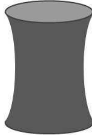
Figure 6.18: Shape of the sample after applying the pressure ( 100\text{ MPa} , then 200\text{ MPa} , then 300\text{ MPa} during 30 min for each) at room temperature. Initial density 71.74\%
