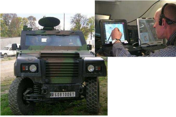
Fig. 1. ISTAR vehicle and its operator, managing video feedback from a UAV and reporting environment activity in the battle management system.
