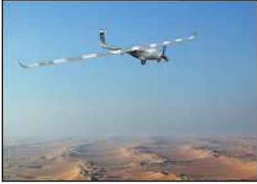
Fig. 1. This long endurance autonomous UAV can perform network relaying or/and observation missions. In both cases, network access in several frequency bands is a critical problem.
