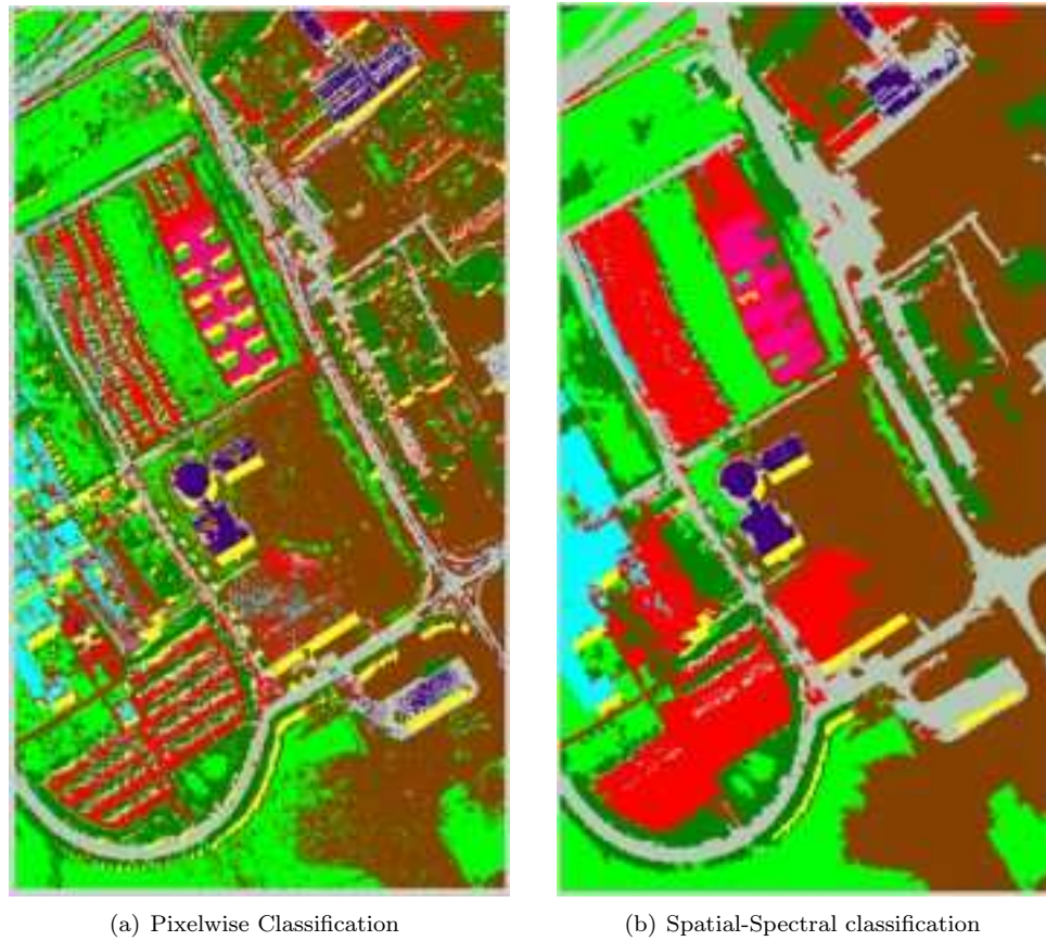
Figure 1.5: Pixelwise and spatial-spectral classification. The aim of spatial-spectral approaches is integrating contextual spatial information with spectral information to produce more "real" results in the classification stage.
