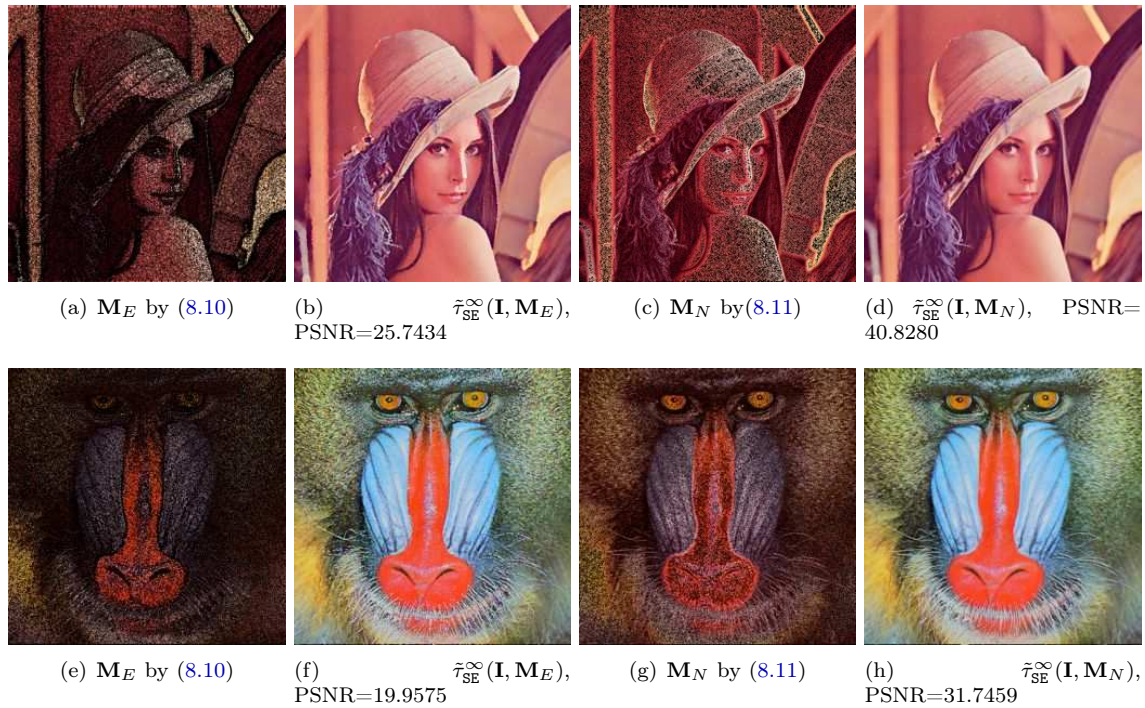
Figure 8.8: Comparison in free-noisy scenario. Conditional toggle mapping handled with different image processing problem according to the mask \mathbf{M} . Particular cases of \mathbf{M} = \mathbf{M}_E as Eq. (8.10) provide edge enhancement (second column) or \mathbf{M} = \mathbf{M}_N as Eq. (8.11) produce an image simplification (fourth column). Masks are computed marginally and displayed as black pixels.
