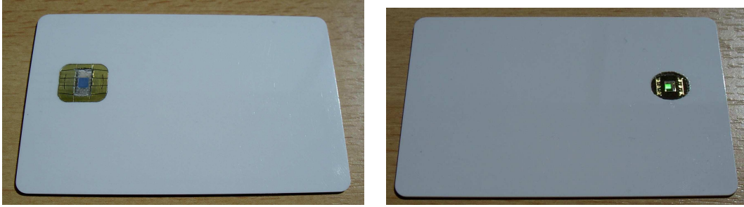
Figure 2.1: Depackaged smart card: back side (left) and front side (right)
