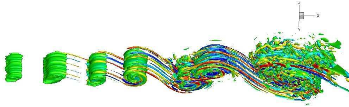
Figure 5.1: Total vorticity field of the three-dimensional coflow mixing layer ([105]). View of an isosurface of the Q -criterion at the value 10^{-5} colored with the streamwise vorticity (levels between \pm 10^5 /s).
