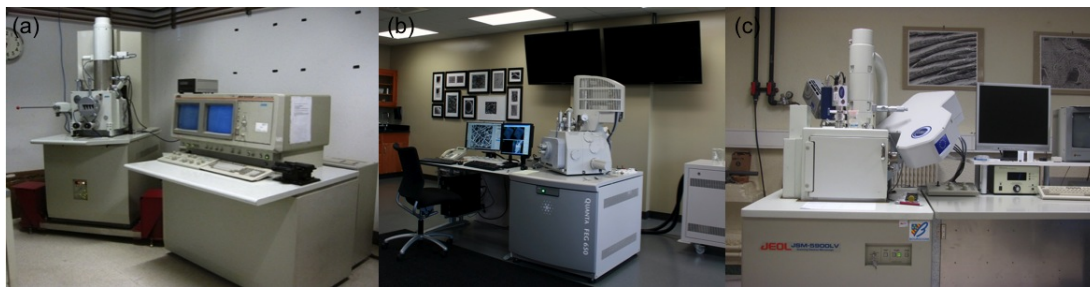
Figure 2.9: Pictures of (a) a JEOL JSM-6400F [171] (ICB, Dijon, France), (b) a FEI Quanta 650 [172] (UAB, Birmingham, AL USA), and (c) a JEOL JSM-5900LV (LaBoMaP, Cluny, France). The JEOL JSM-5900LV is equipped with an Oxford INCA x-act EDS/WDS system.
