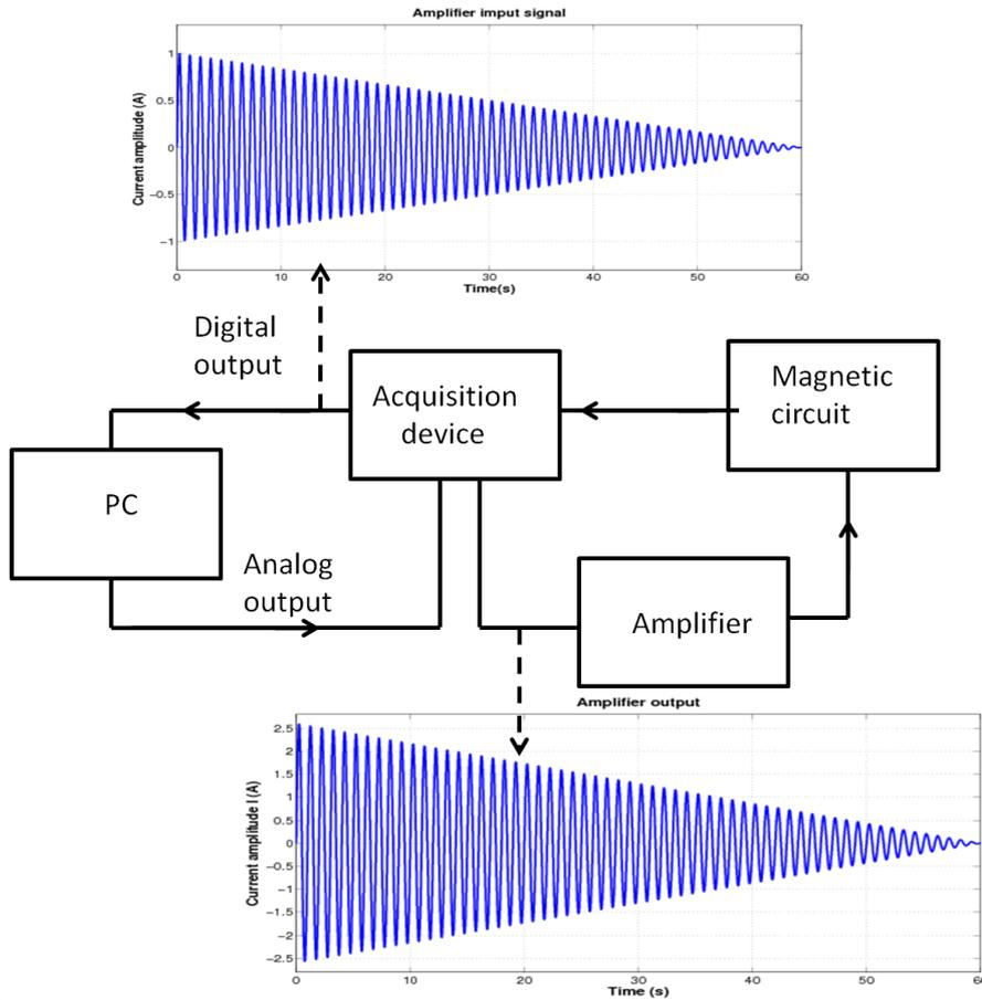
Figure 2.38 – Degaussing block diagram.
