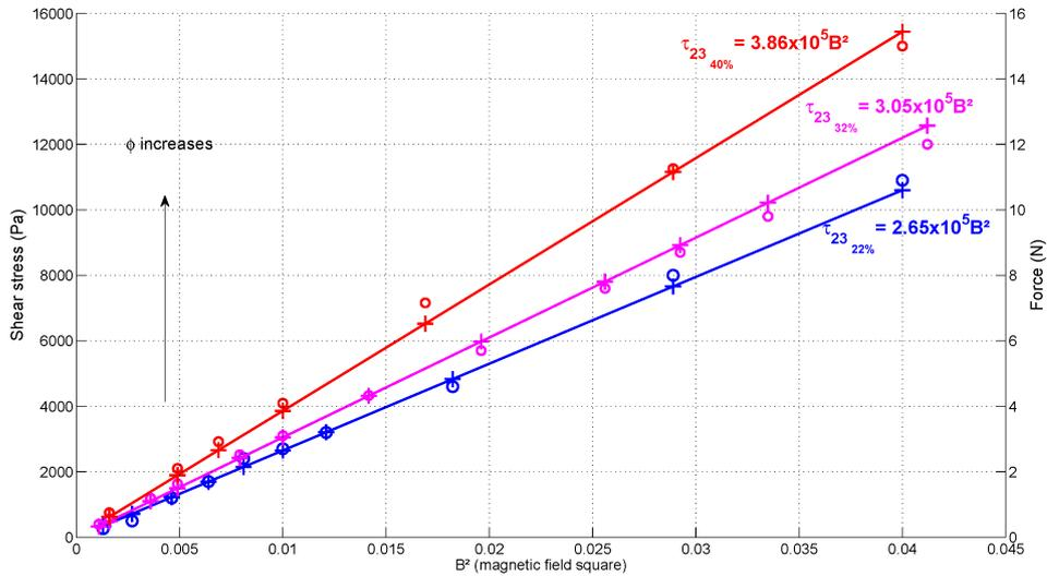
Figure 6.4 – Variation of the  $\tau_{23}$  as a function of  $B^2$  for different MRF particle volume fractions. Blue:  $\phi=0.22$ . Magenta:  $\phi=0.32$ . Red:  $\phi=0.4$ . Shearing with an non-magnetic shearing plate (the corresponding forces also indicated).
