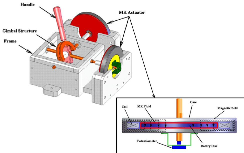
Figure 1.10 – MRF joystick (after W.H.Li et al., [40]).
