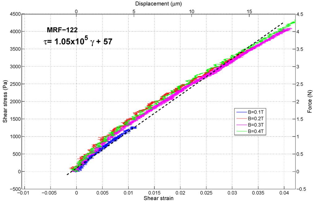
Figure 4.13 – Shear stress as function of shear strain (also indicated force and displacement) for magnetic field values between  $0.1$  T and  $0.4$  T at a shear rate  $\dot{\gamma} = 0.02$  s<sup>-1</sup>.
