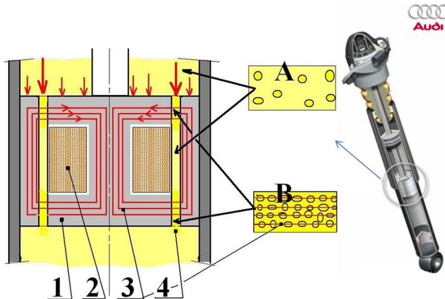
Figure 1.7 – Audi magnetic ride; 1:valve 2:coil 3:magnetic field 4:MRF (after [www.audi.com](http://www.audi.com)).
