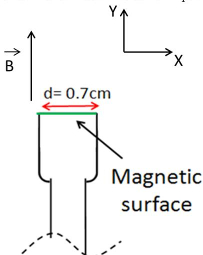
Figure 3.8 – Schematic representation of the external permanent magnet.
