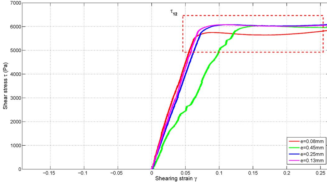
Figure 4.25 – Variation of  $\tau_{12}$  with shearing plate thickness.
