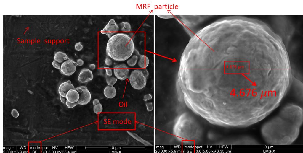
Figure 3.4 – SEM of a) MRF aggregate b) isolated MRF particle (see the scale at the lower right corner of the picture).
