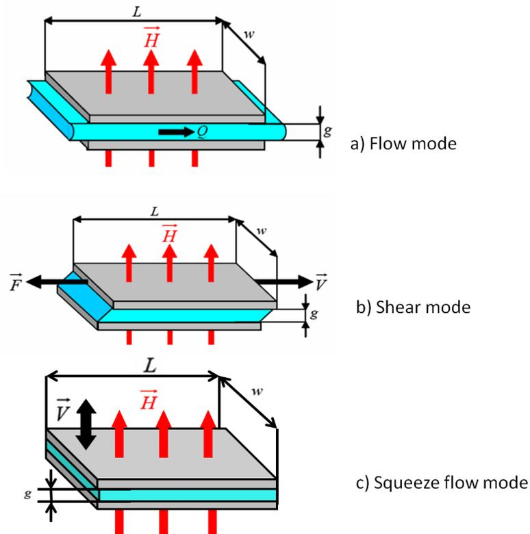
Figure 1.5 – Basic operational modes of MRF.
