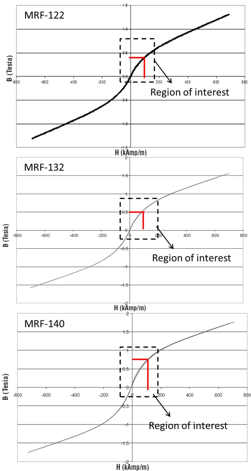
Figure 1.30 – Typical magnetic properties for Lord MRFs [10].
