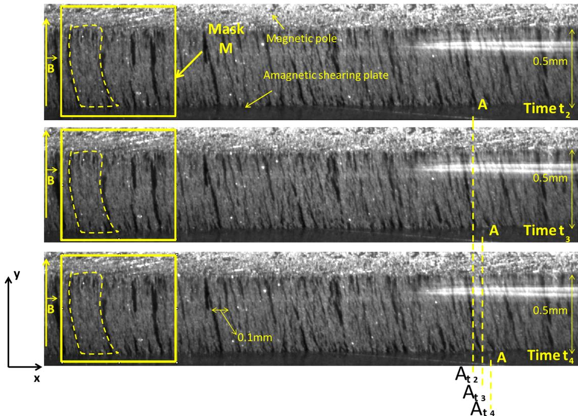
Figure 3.27 – MRF internal structure during loss of adhesion with the amagnetic shearing plate. (Top to bottom corresponds to the succession of the shearing moments with a time interval equal to  $\Delta t=10s$ ).
