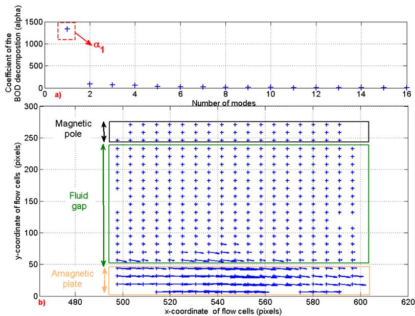
Figure 3.28 – BOD of the MRF shearing with an amagnetic plate in the no adhesion phase; top figure: eigen values  $\alpha$  of the BOD decomposition; bottom figure: cartesian coordinates of the velocity in the  $\alpha_1$  mode.
