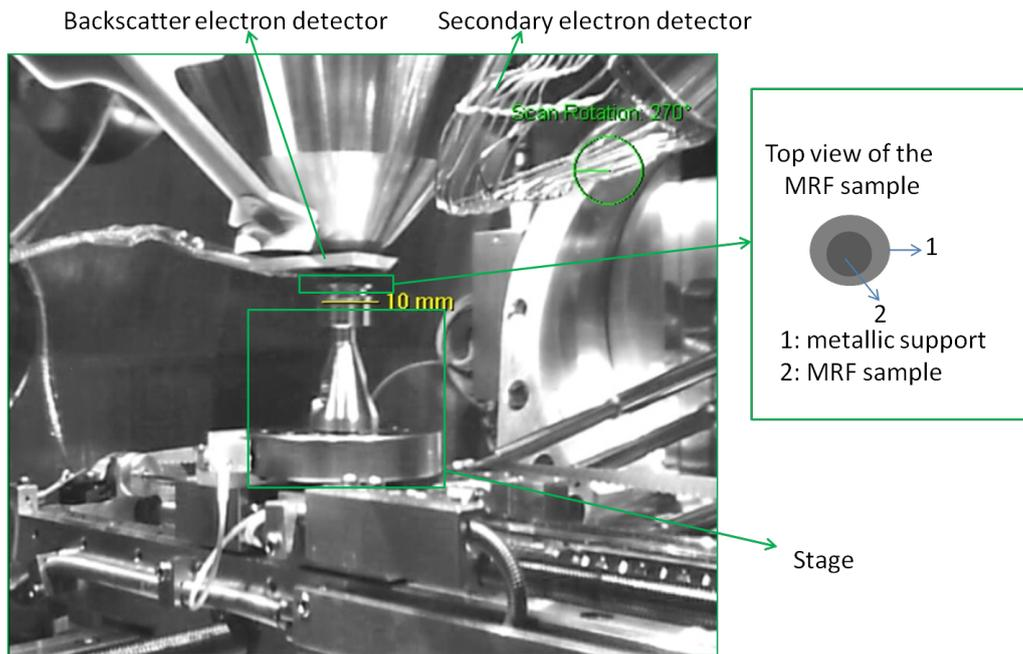
Figure 2.19 – Internal view of the SEM chamber.
