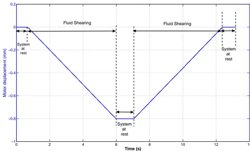
Figure 2.14 – Typical displacement imposed by the motor.
