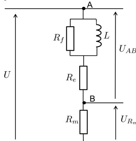
Figure 2.10 – Equivalent electric network of the coils.
