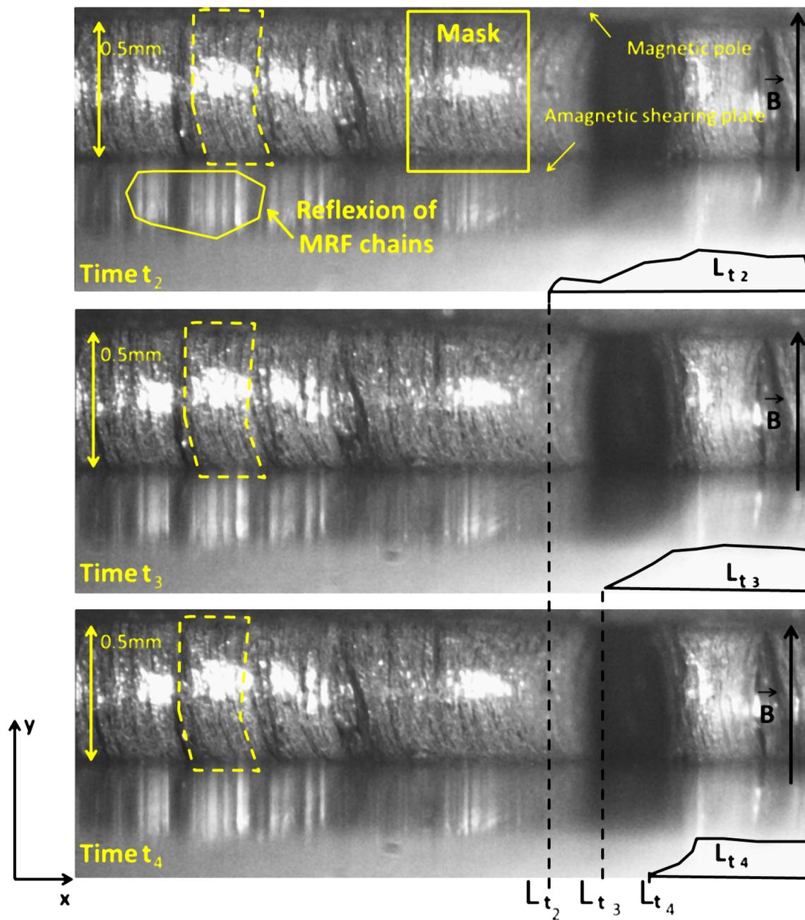
Figure 3.29 – MRF internal structure during loss of adhesion with an amagnetic plate (Top to bottom corresponds to the succession of the shearing moments with a time interval equal to  $\Delta t=55\text{s}$ ).
