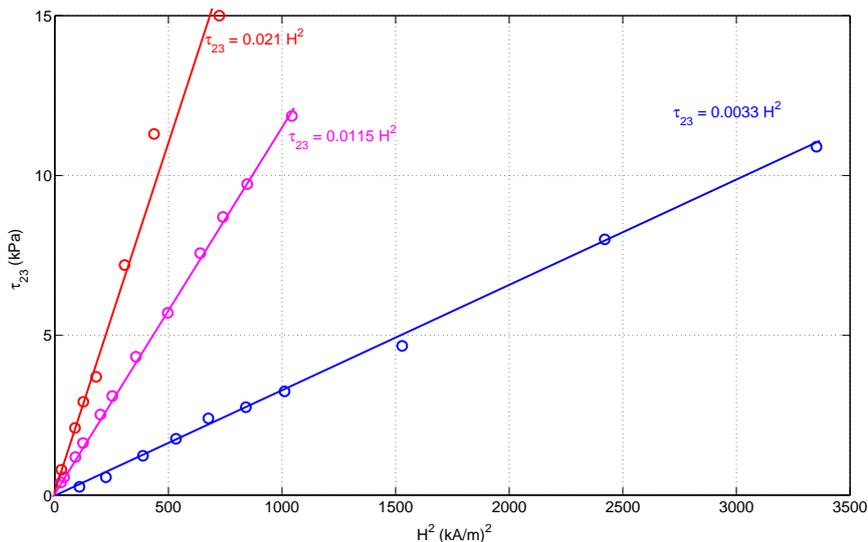
Figure 6.5 – Variation of the maximum shear stress as function of the square of the applied magnetic field  $H^2$  with MRF particle volume fraction : blue curves:  $\phi=0.22$ ; magenta curves:  $\phi=0.32$ ; red curves:  $\phi=0.4$  when shearing with an amagnetic shearing plate.
