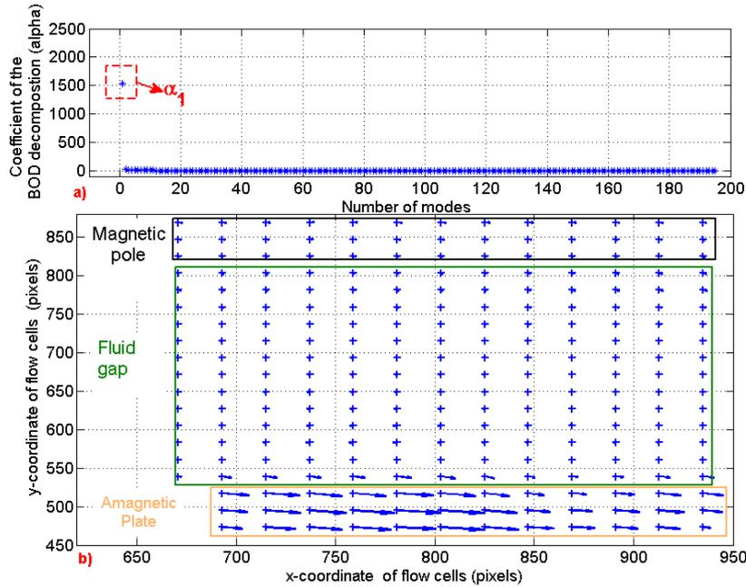
Figure 3.30 – BOD of the MRF shearing with an amagnetic plate in the no adhesion phase; top figure: eigen values  $\alpha$  of the BOD decomposition; bottom figure: cartesian coordinates of the velocity in the  $\alpha_1$  mode.
