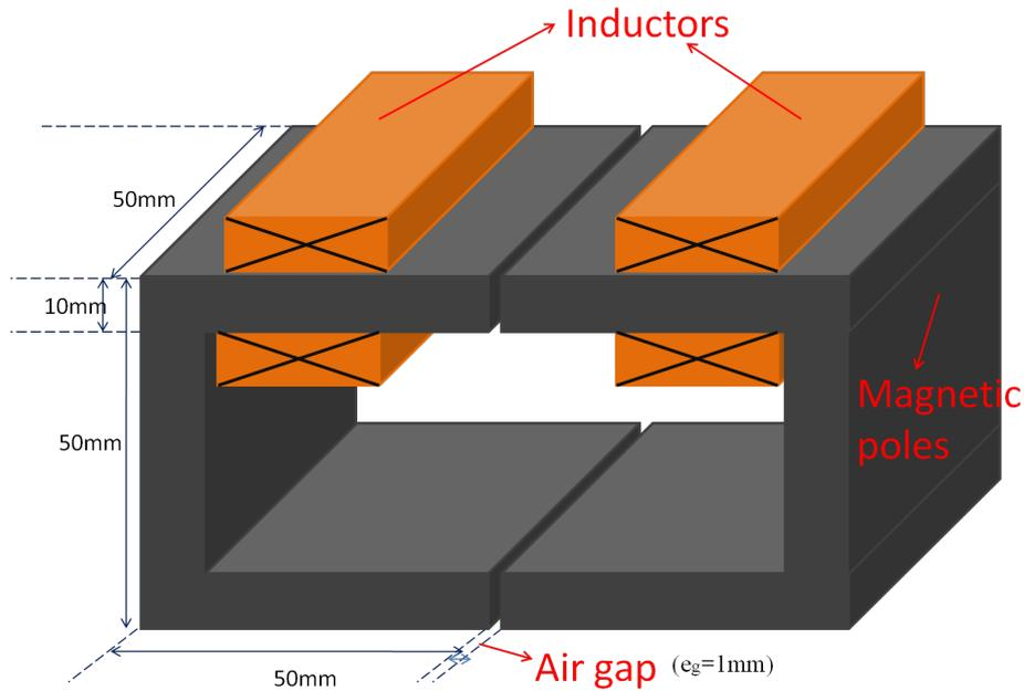
Figure 2.11 – Three dimensional view of the magnetic pole.
