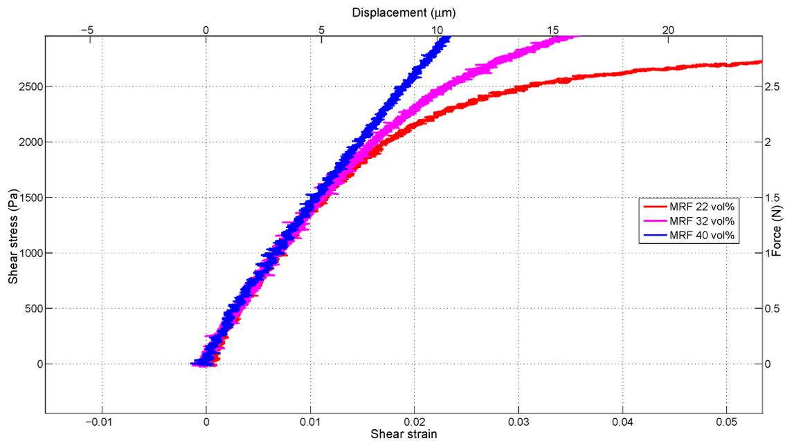
Figure 4.15 – Variation of shear stress as function of shear strain (also indicated force and displacement).
