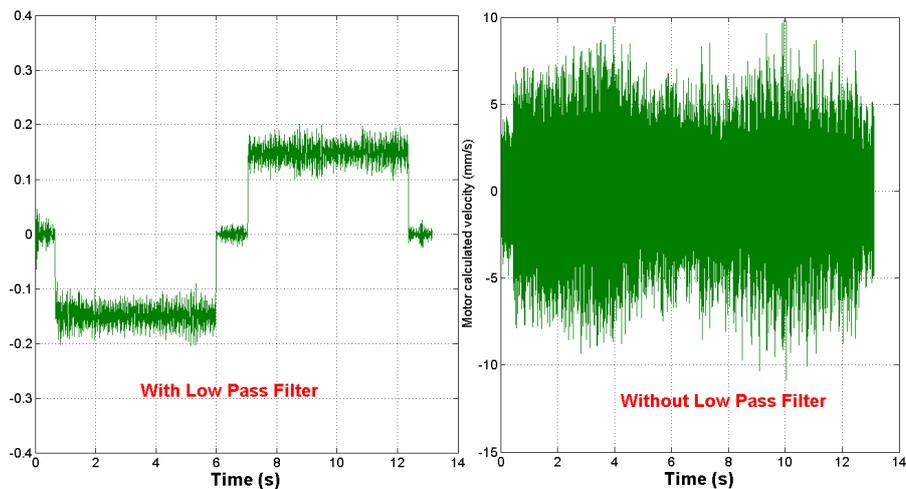
Figure 2.33 – Velocity profile with and without digital filtering.
