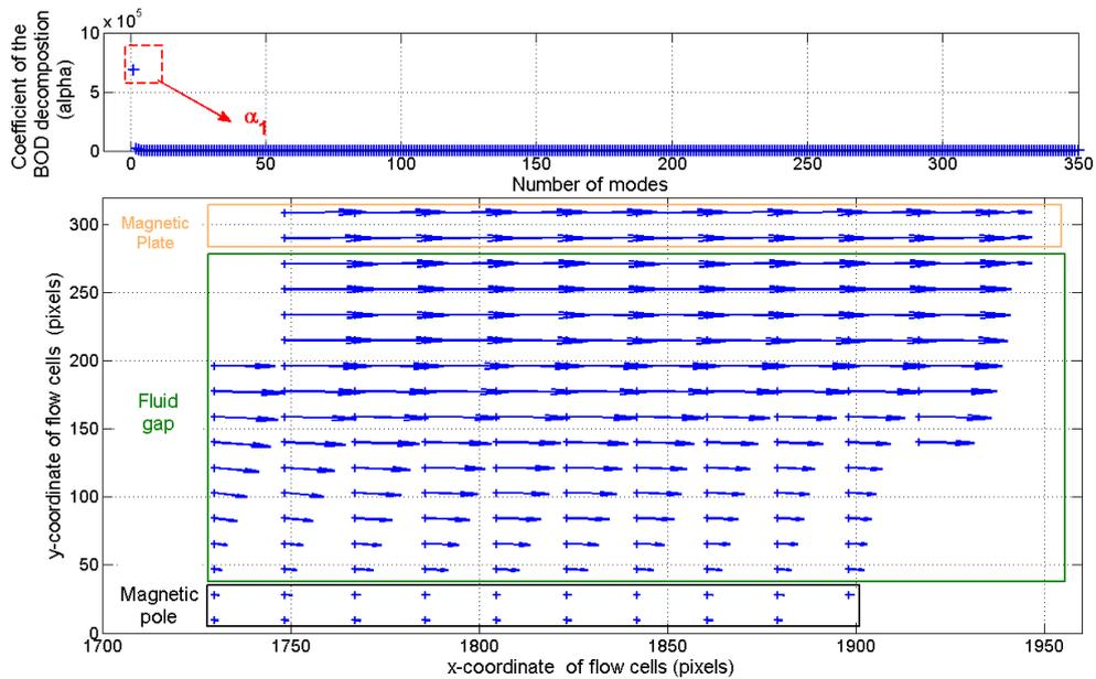
Figure 3.32 – BOD of the MRF shearing phase with a magnetic plate in the "No adhesion phase". Top figure: eigen values  $\alpha$ ; bottom figure: cartesian coordinates of the velocity in the  $\alpha_1$  mode.
