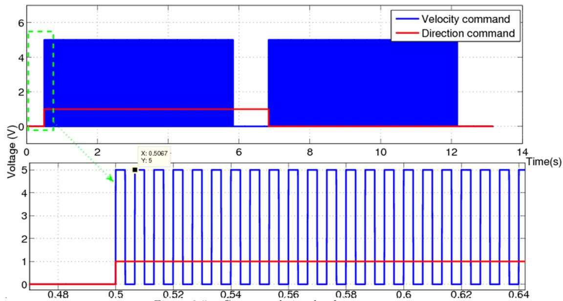
Figure 2.5 – Command signals of stepper motor.
