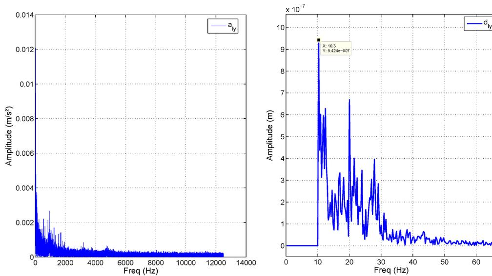
Figure 2.30 – Plate support vibrations in the  $y$  and  $z$  directions; left:acceleration right:displacement.
