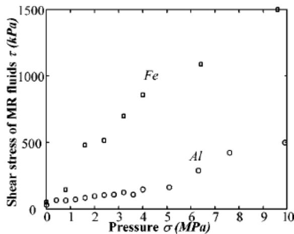
Figure 1.27 – Comparison between different work pieces shear stress response ( $B=275$  mT). (after Zhang et al.,[54]) Fe: iron test slice; Al: Aluminum test slice.
