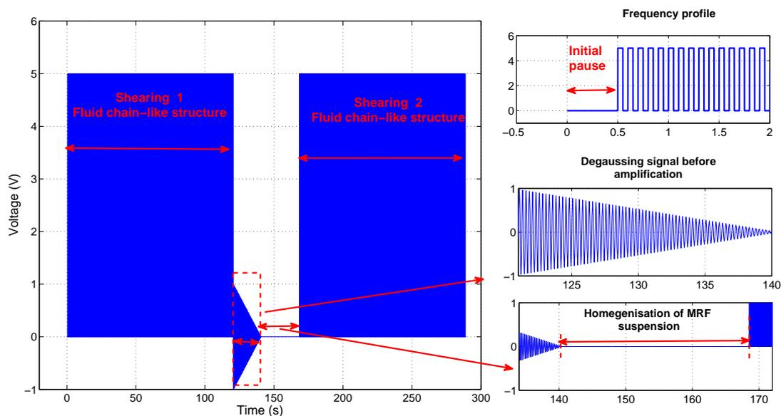
Figure 4.7 – Shearing command for the succession of experimental measurements.
