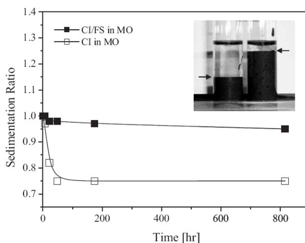
Figure 1.4 – Comparison between sedimentation ratio of carbonyl iron (CI) and carbonyl iron fumed silica mixture (CIFS) in mineral oil solution (MO) (after Sung et al.,[49]).
