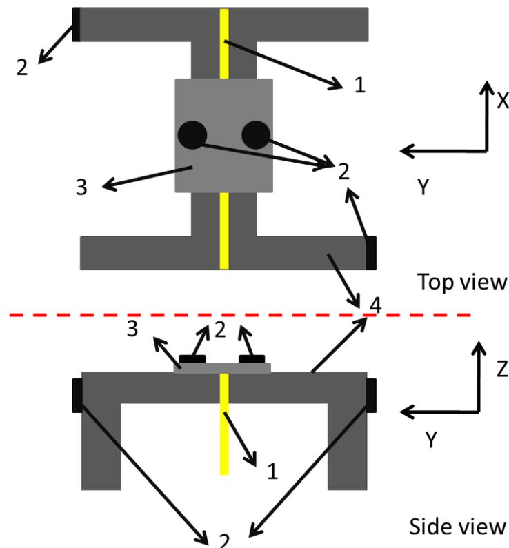
Figure 2.31 – Top and side view of plate support with fixed tests accelerometers: 1: plate; 2: accelerometers; 3: thick aluminum plate; 4: plate support.
