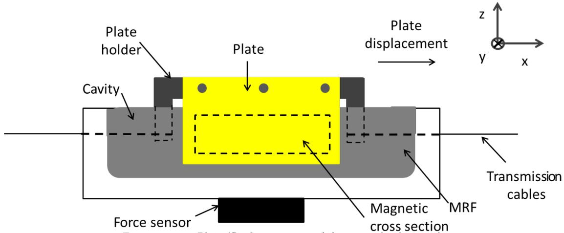
Figure 2.15 – Plate/fluid cavity view (after www.kistler.com).
