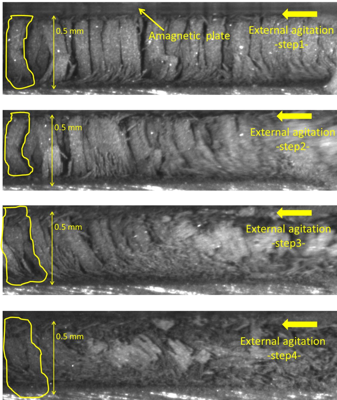
Figure 3.17 – Destruction of MRF internal chain structure.
