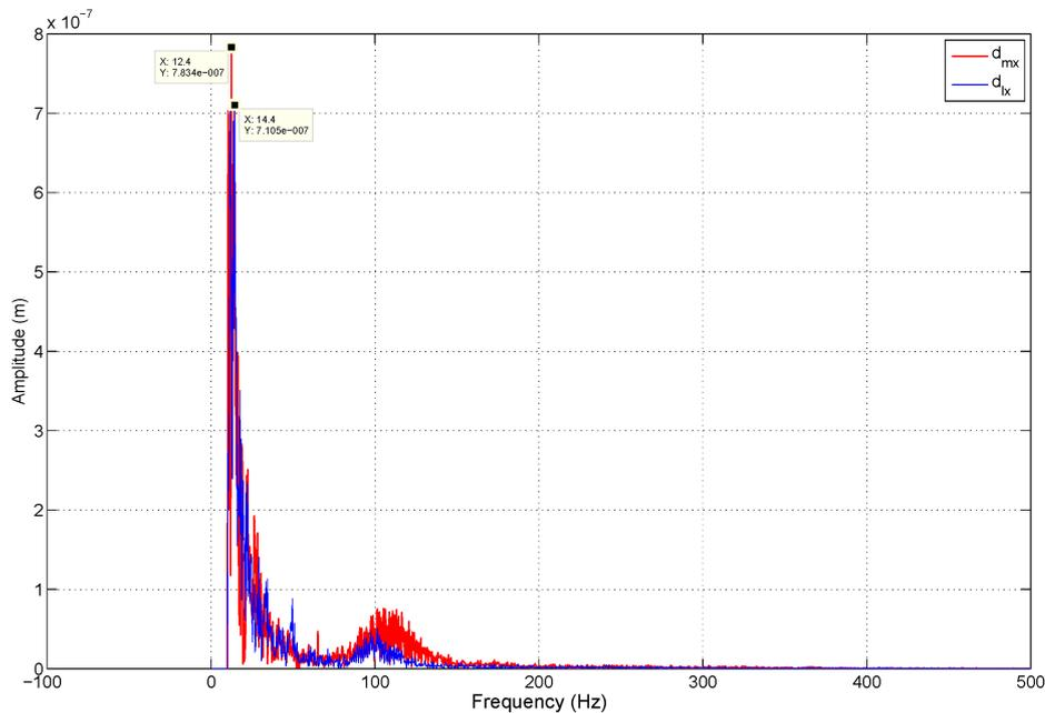
Figure 2.27 – Motor and plate holder displacement measurement.
