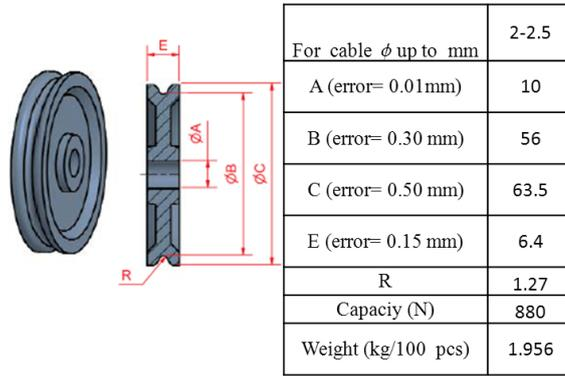
Figure 2.9 – Pulley structure.
