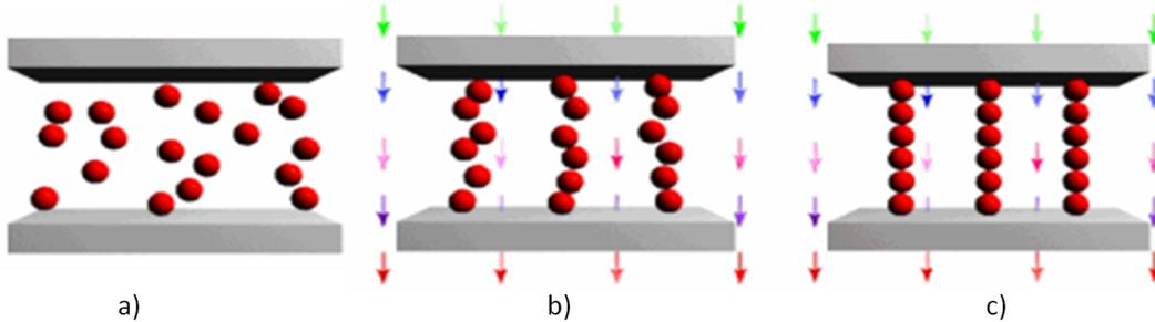
Figure 1.1 – Activation steps of MR fluid, arrows present the magnetic field  $B$  direction (after Fernando Goncalves [20]).
