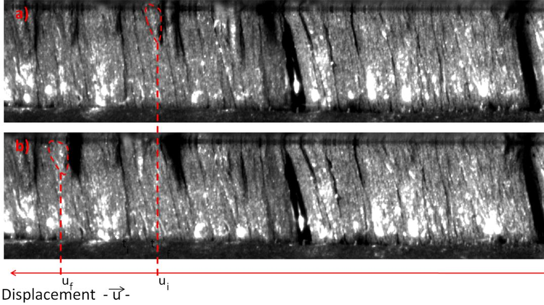
Figure 6.16 – Example of the MRF-132 internal structure in the sliding regime.
