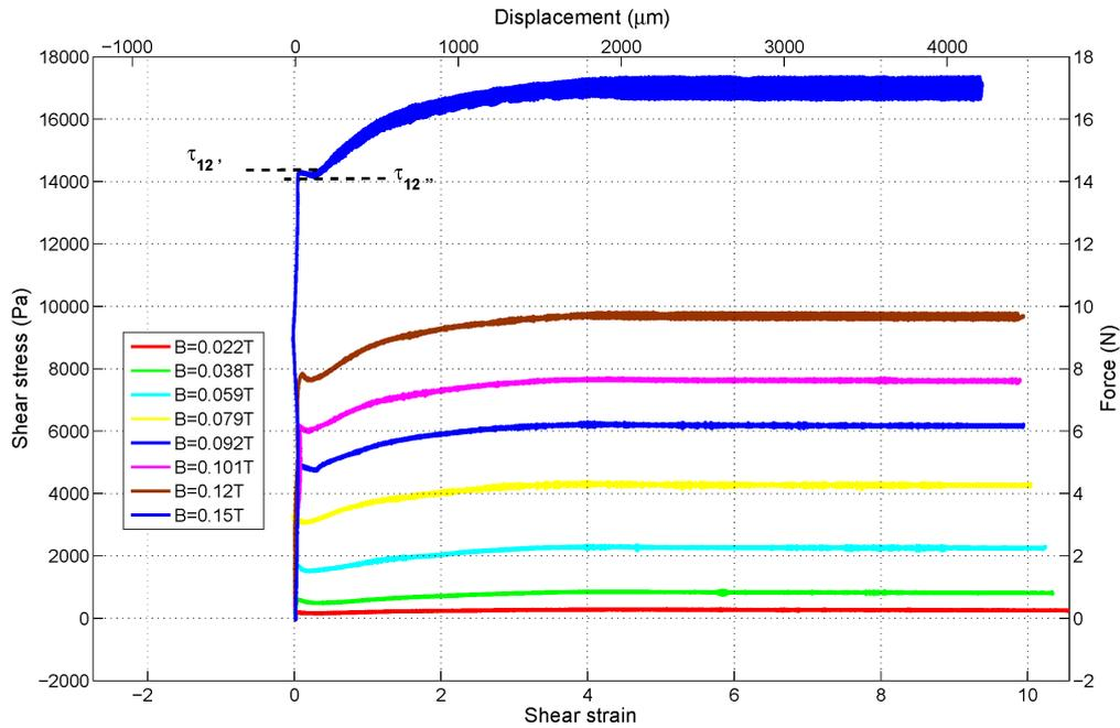
Figure 4.19 – Shear stress as function of the shear strain (also indicated: force and displacement) resulting from shearing with a magnetic plate.
