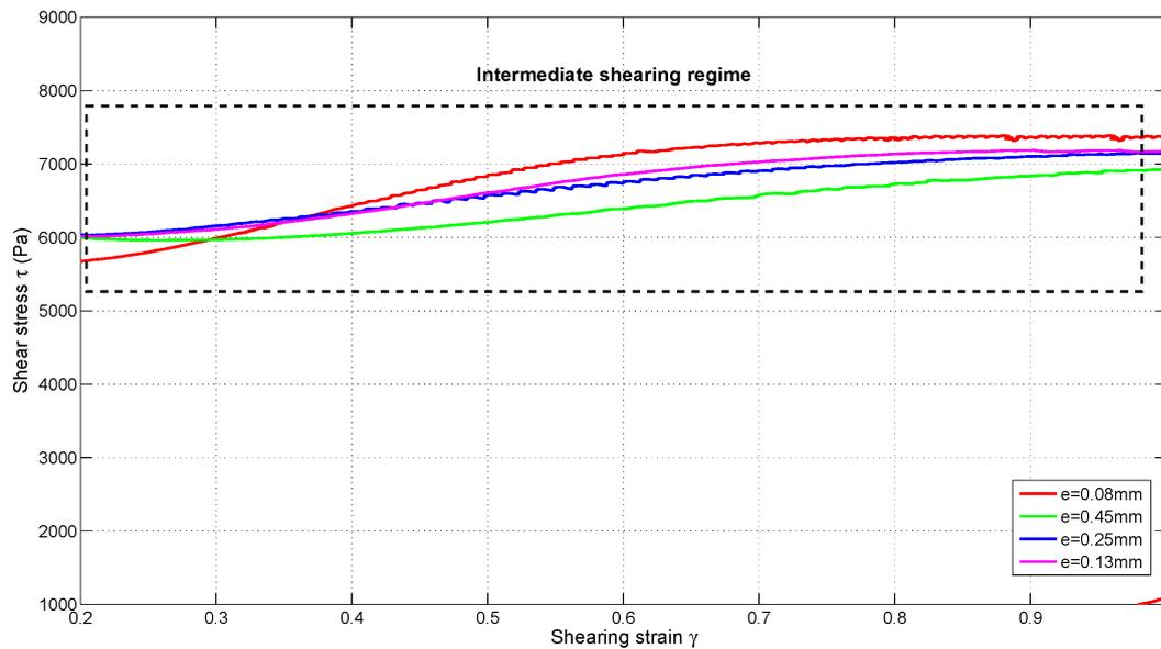
Figure 5.8 – Dependency of  $\tau(\gamma)$  with shearing plate thickness in the intermediate shearing.
