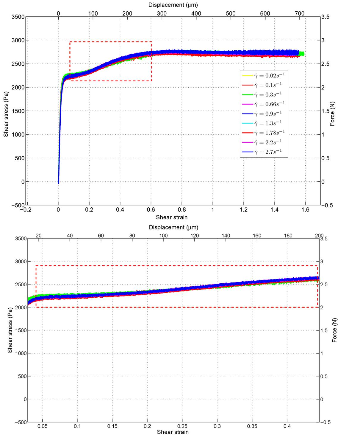
Figure 5.1 – Mean shear stress as a function of the mean shear strain (averaged over the fluid shearing gap  $g_f$ ). Shearing with an amagnetic plate at different shearing velocity values (also indicated force and displacement). Top: total fluid response; bottom: highlight of MR fluid response in regime 2.
