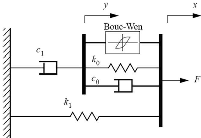
Figure 1.33 – Modified Bouc-Wen model for MRF after [1]
