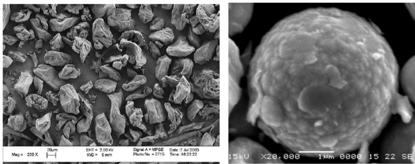
Figure 1.3 – SEM photograph of a) guar gum powder; b) cast iron particle coated with guar gum (after Fang et al.,[14]).
