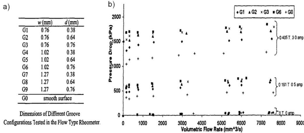
Figure 1.26 – Effect of groove configuration on the measured pressure drop force (after Gordaninejad et al.,[24]).
