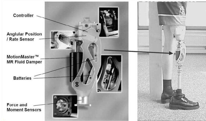
Figure 1.9 – Commercial "Smart Magnetix" prosthesis provided by a MotionMaster MR fluid damper (after J. David Carlson [7]).
