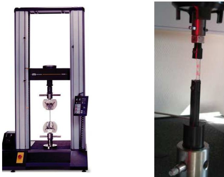
Figure 1: Left: The Instron equipment. Right: Design of specific clamps. Specimens were dotted for video extensometer recognition.
