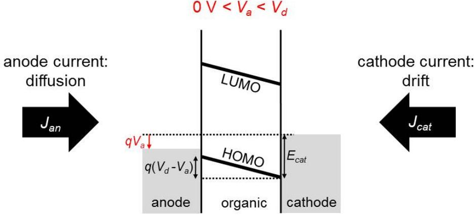
Figure 4.13: Energy diagram of an MIM organic diode under small forward-bias  $V_a$ . An analytical current-voltage model is developed here by only considering the dominant current mechanism at each contact side; diffusion current from the anode and drift current from the cathode.
