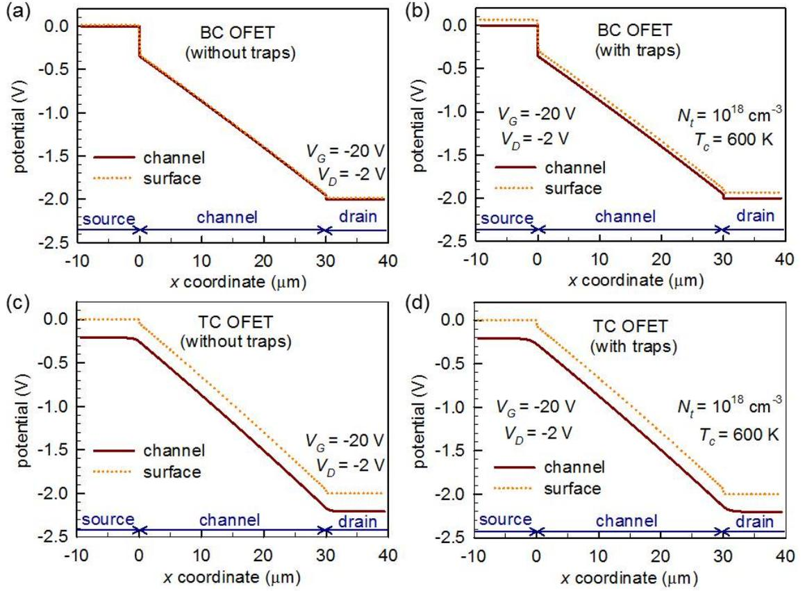
Figure 5.11: Simulated potential profiles in BC/TC OFETs with/without existence of trap states. Upon the assumption of the equipotential channel at  $V_D = 0$  V, all extracted potential profiles are corrected with the reference profile at  $V_D = 0$  V.
