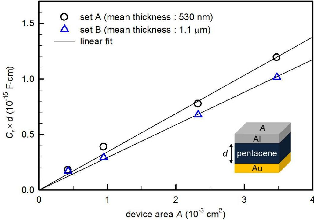
Figure 4.8: Experimental method for estimating quasi-static dielectric constant. The slope of the linear fit corresponds to  $k\epsilon_0$  by Equation (4.2). Inset: MIM capacitance with the geometrical dimensions.
