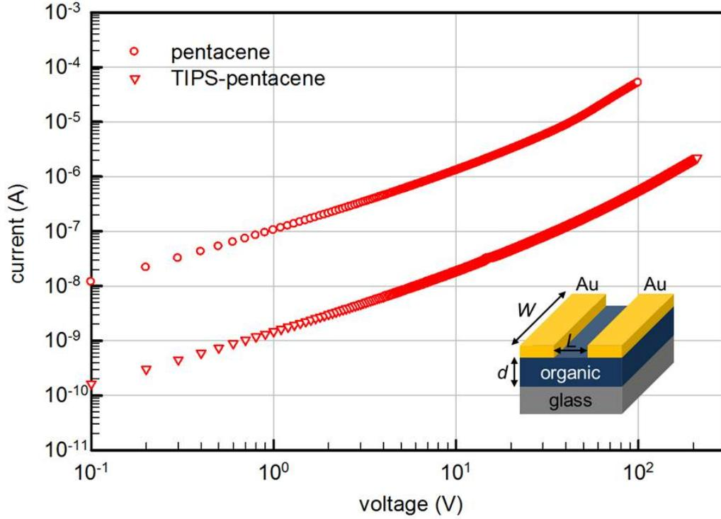
Figure 4.27: Current-voltage characteristics of pentacene and TIPS-pentacene gap-type diodes drawn on a log-log plot. The inset is the schematic device structure.
