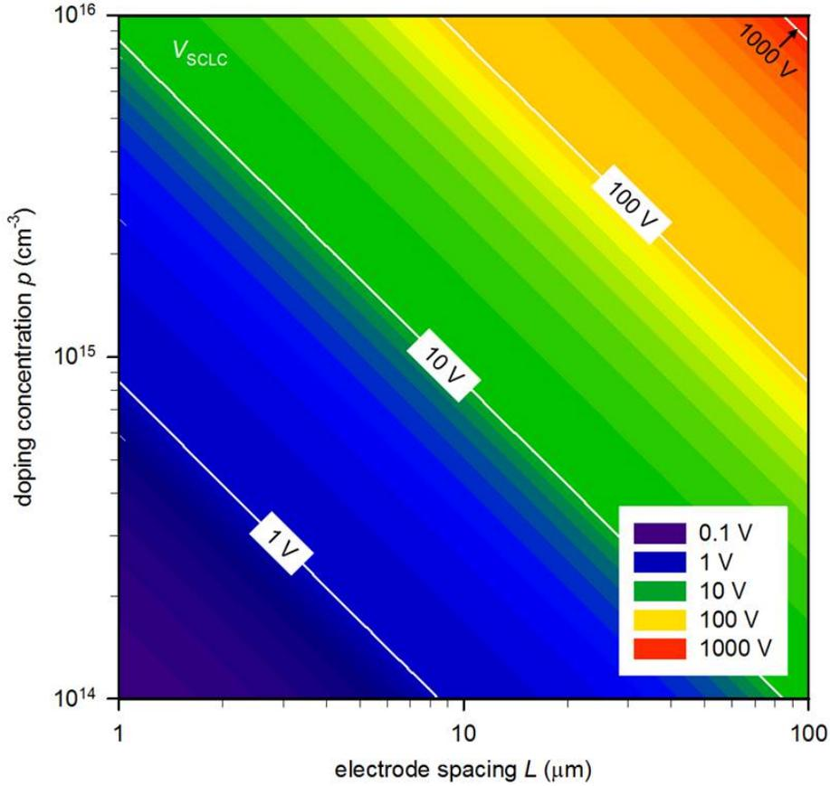
Figure 4.32: The SCLC onset voltage  $V_{\text{SCLC}}$  calculated by Equation (4.44) for expecting the operation regime of an organic gap-type diode. Fixed parameters are  $d=150$  nm and  $\epsilon_s = 3.6 \times \epsilon_0$ .
