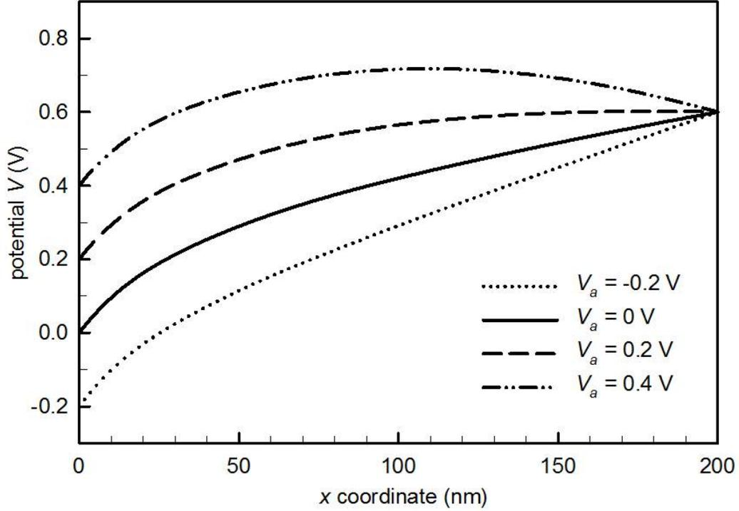
Figure 4.17: Potential profiles obtained by the numerical simulation under different bias conditions. The variation of the effective  $\Delta V$  is the evidence for the trap-induced ideality factor in the low-voltage regime.
