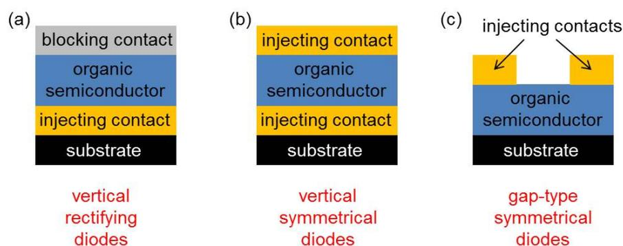
Figure 4.1: Illustration of the different diode structures.
