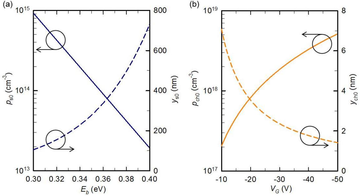
Figure 5.15: (a) Source distribution factors ( $p_{s0}$  and  $y_{s0}$ ) as a function of  $E_b$  and (b) channel distribution factors ( $p_{ch0}$  and  $y_{ch0}$ ) as a function of  $V_G$ . The solid lines indicate the initial hole concentrations and the dashed lines correspond to the distribution lengths.
