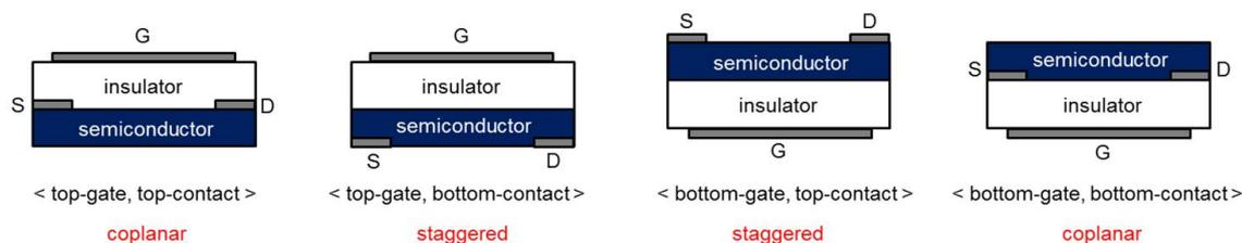
Figure 5.9: Four possible OFET geometries depending on the relative positions of the gate (G) and the source/drain (S/D) electrodes.
