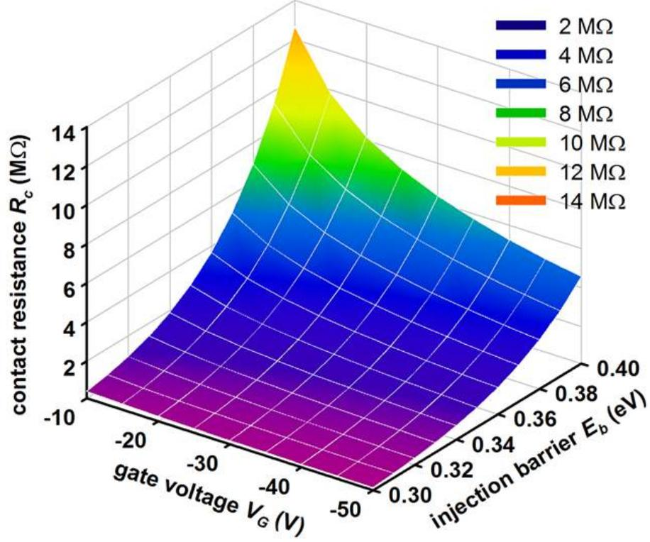
Figure 5.17:  $R_c$  determined by Equation (5.35) with a variation of  $V_G$  and  $E_b$ . The fixed parameters are as follows;  $N_v = 10^{20} \text{ cm}^{-3}$ ,  $T = 300 \text{ K}$ ,  $\epsilon_s = 3.6 \times \epsilon_0$ ,  $C_i = 2.3 \text{ nF/cm}^2$ ,  $V_T = 0 \text{ V}$ ,  $d = 50 \text{ nm}$ ,  $W = 500 \mu\text{m}$ , and  $\mu = 0.2 \text{ cm}^2/\text{V}\cdot\text{s}$ .
