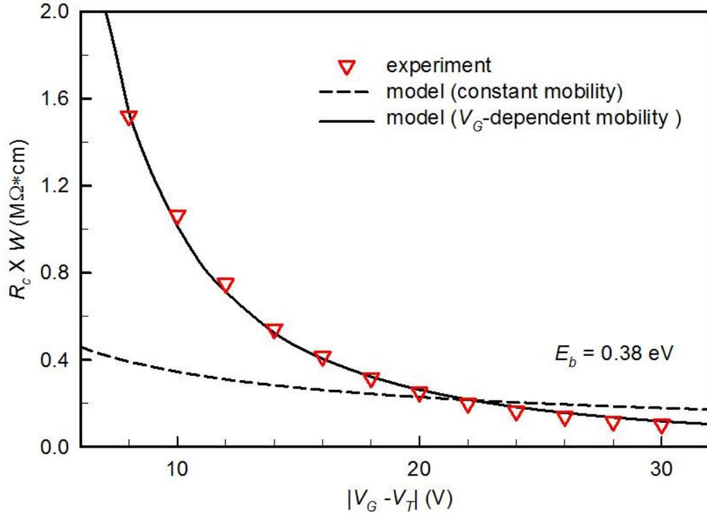
Figure 5.21: TLM-extracted  $R_c W$  as a function of  $|V_G - V_T|$  in comparison to the charge-based  $R_c$  model. Note that, if a constant mobility is assumed (here  $0.2 \text{ cm}^2/\text{V}\cdot\text{s}$ ), the  $V_G$ -dependence of  $R_c$  is underestimated. When we take the  $V_G$ -dependent mobility into account, the experimental results could be well fitted by the model.
