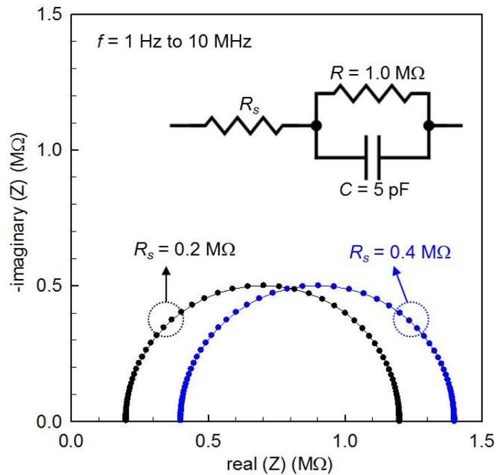
Figure 3.4: Complex-plane representation of the simulated impedance spectra of the circuit in the inset with different series resistance  $R_s$  values. Simulation frequency points are from 1 Hz to 10 MHz with 20 points per decade.
