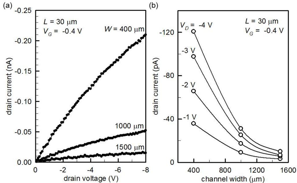
Figure 5.8: Effect of the channel length  $W$  on  $I_D$ . (a) Output characteristics of three OMESFETs with  $L=30 \mu\text{m}$  and different  $W$  values. (b) Variation of  $I_D$  as a function of  $W$ .
