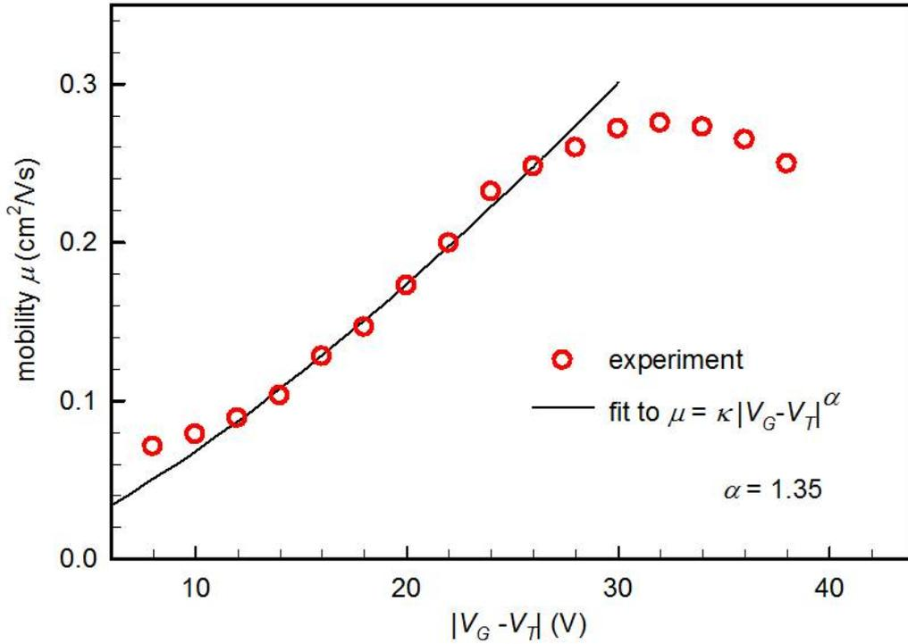
Figure 5.20: Hole mobility as a function of  $|V_G - V_T|$  extracted by the TLM. The solid line is a fit to the trap-filling model at low  $|V_G|$ . The decrease in the mobility at higher  $|V_G|$  can be attributed to the field-induced mobility degradation.
