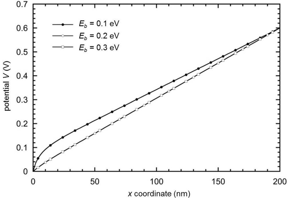
Figure 4.12: Potential profiles along the semiconductor thickness calculated by the model Equation (4.15). The profiles are practically straight as long as the injection barrier is not too small.
