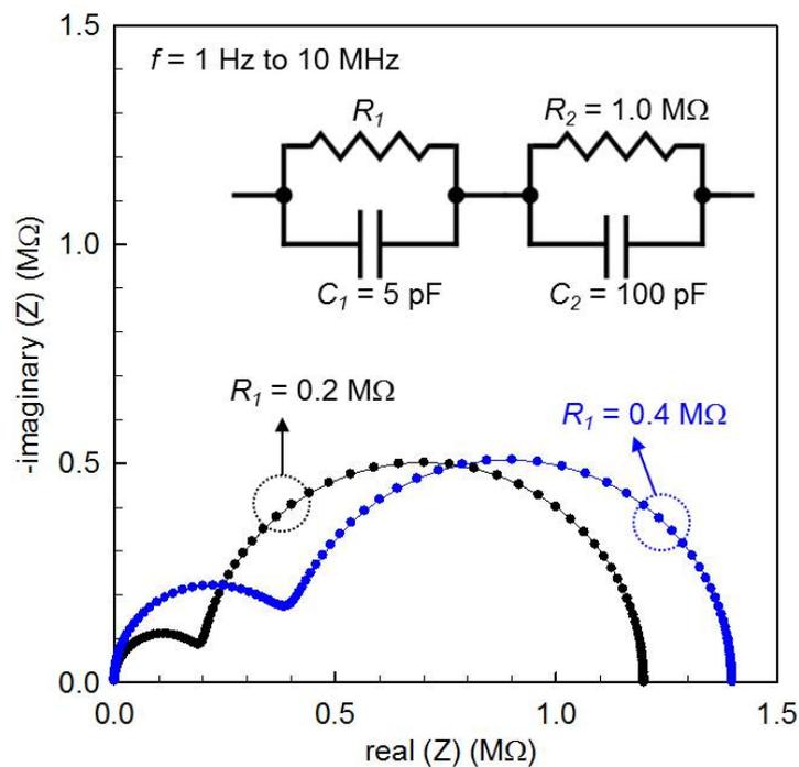
Figure 3.5: Complex-plane representation of the simulated impedance spectra of the circuit in the inset with different  $R_1$  values. Simulation frequency points are from 1 Hz to 10 MHz with 20 points per decade.
