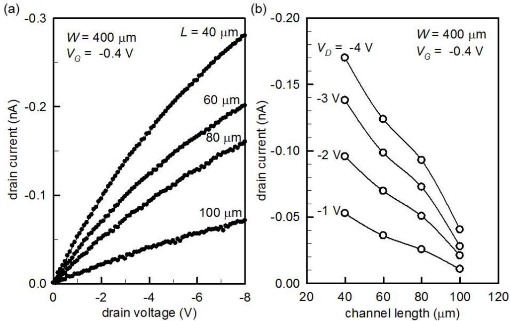
Figure 5.7: Effect of the channel length  $L$  on  $I_D$ . (a) Output characteristics of four OMESFETs with  $W=400 \mu\text{m}$  and different  $L$  values. (b) Variation of  $I_D$  as a function of  $L$ .
