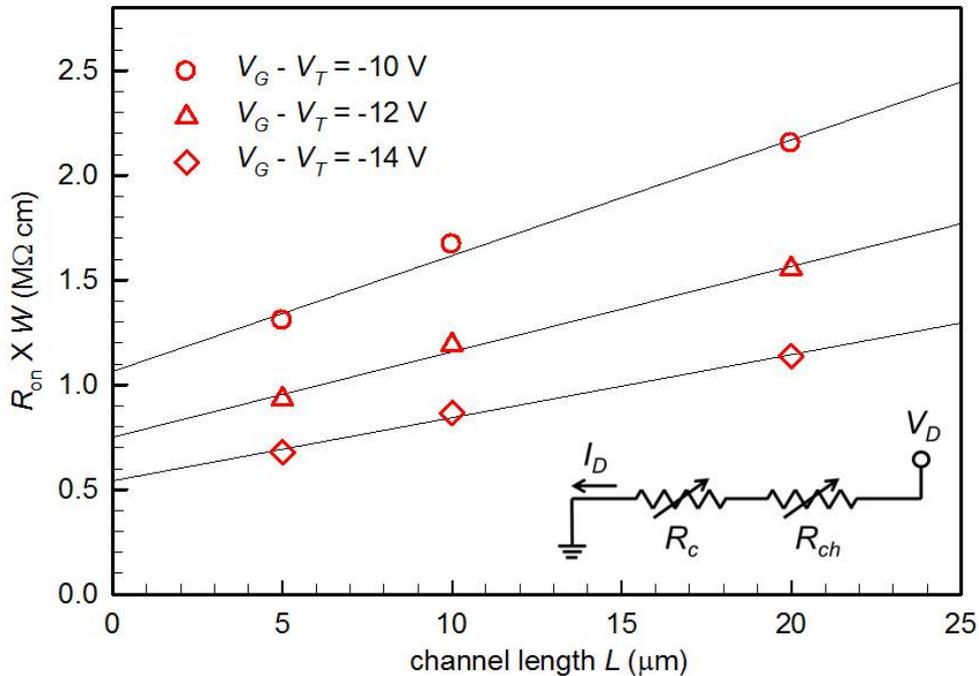
Figure 5.19:  $R_{on}W$  versus  $L$  plot for the transmission-line method (TLM). The inset is the equivalent circuit of the on-state conduction path that consists of a series connection of the contact and channel resistances. Note that  $R_c$  and  $R_{ch}$  are drawn as variable resistors because both of them are supposed to be  $V_G$ -controlled.
