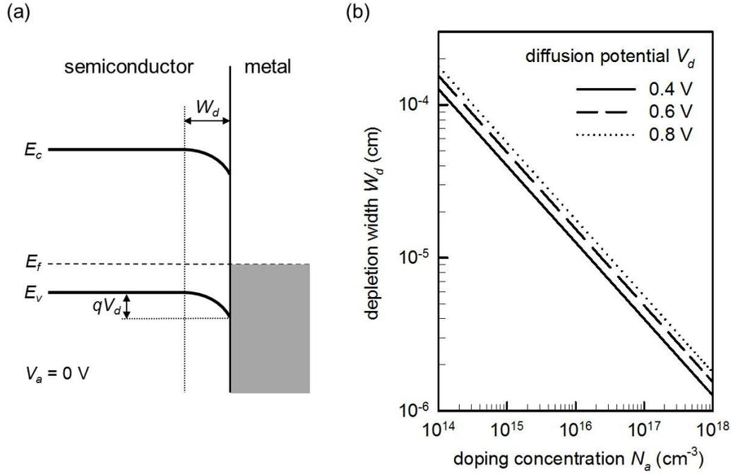
Figure 4.2: (a) Energy band structure at a metal/p-type semiconductor interface at thermal equilibrium ( $V_a = 0$  V).  $E_c$ : conduction band edge,  $E_v$ : valence band edge, and  $E_f$ : Fermi level. (b) Calculated depletion width as a function of doping density at several diffusion potential values.
