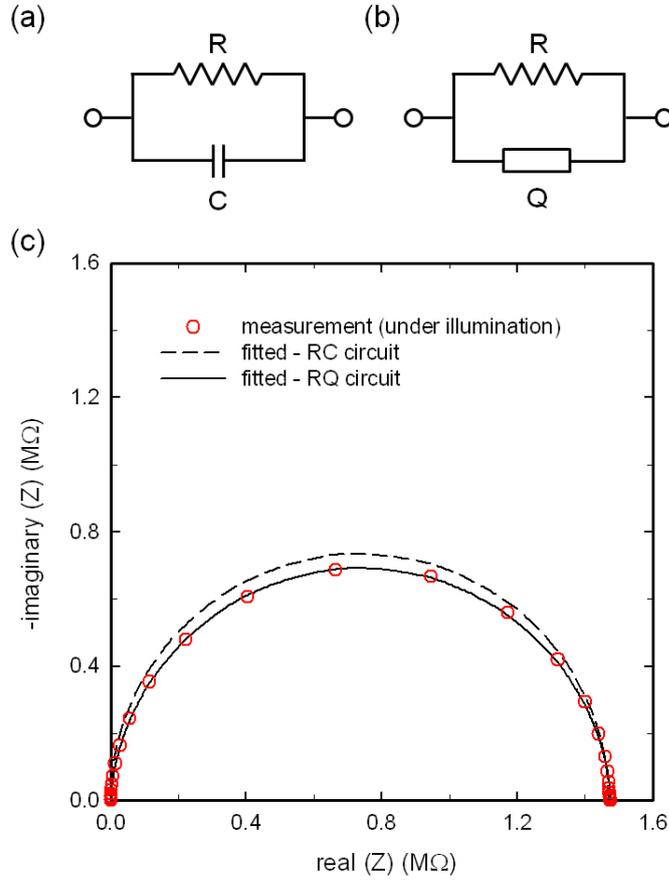
Figure 4.24: (a) Parallel resistance and capacitance circuit (RC circuit). (b) Parallel resistance and CPE (constant-phase element) circuit (RQ circuit). (c) Fitted experimental data to both RC and RQ equivalent circuits.
