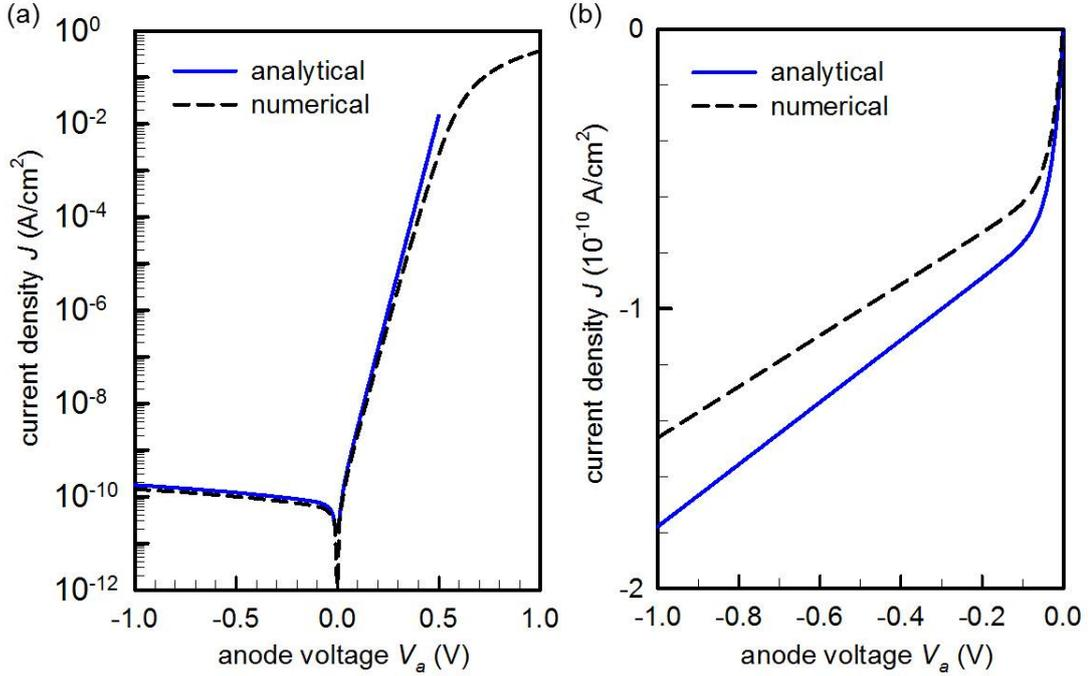
Figure 4.14: Current voltage characteristics for comparing the analytical model with the numerical finite-element simulation. (a) From reverse- to injection-limited regime in semi-log scale. (b) Reverse-bias regime in linear scale.
