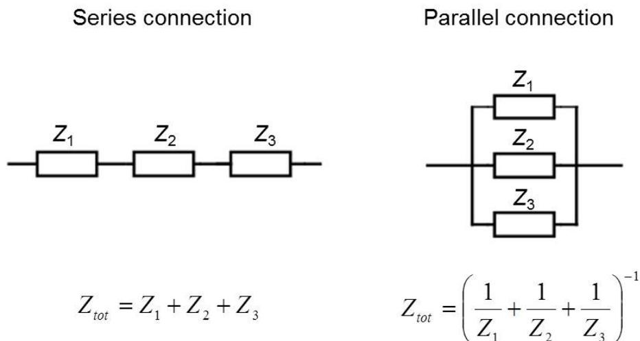
Figure 3.2: Total impedance of a series impedance circuit and a parallel impedance circuit by combination rules.
