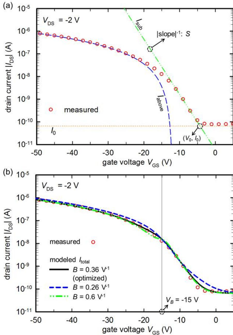
Figure 5.23: (a) A measured linear-regime transfer curve on a semi-logarithmic plot with graphical instructions on the subthreshold parameters. (b) The effect of the transition parameter  $B$  on the final model including below-to-above threshold transition.
