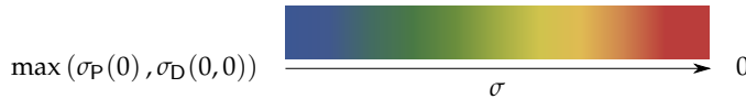
Figure 4.7: Legend for the stress values. Blue correspond to the maximum stress level sustained by the bar while red stands for a vanishing stress
