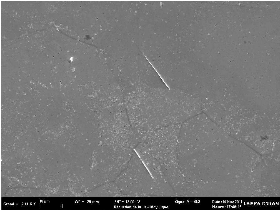
(a) \sigma_a/\tau_a = 2.0, \sigma_a = 68 \text{ MPa}, \beta = 45^\circ
