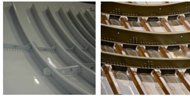
(a) Elementary part made of aluminum skin, stringers and frames (b) Elementary part made of composite materials skin, stringers and frames
