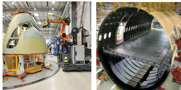
(a) Nose fuselage subsection subjected to robotized drilling operations (b) Fuselage subsection made of composite materials
