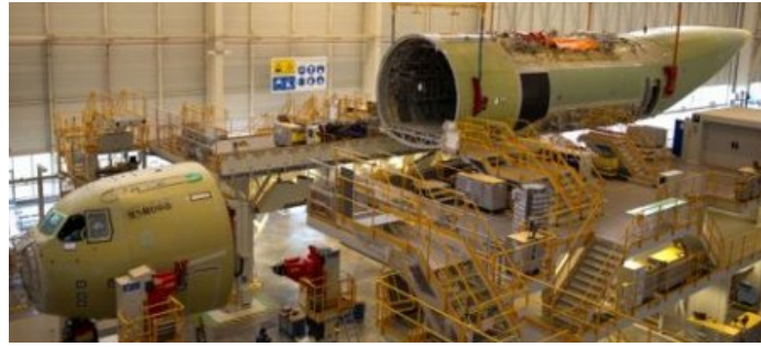
Figure 1.3 – Example of an aeronautical final assembly line (FAL)
