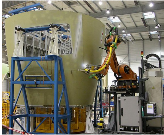
Figure 3.3 – Example of drilling operations being performed by a robot on a large structure presenting different local stiffness levels. Such robots also present different vibratory behaviors as a function of their positioning
