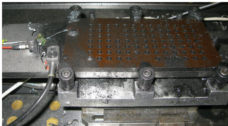
(d) View of the test bed after 88 drillings have been performed: the sample is covered by cutting fluid and CFRP dust mud. Only 68 out of the 88 drillings have been performed with the AE sensor integration apparatus
