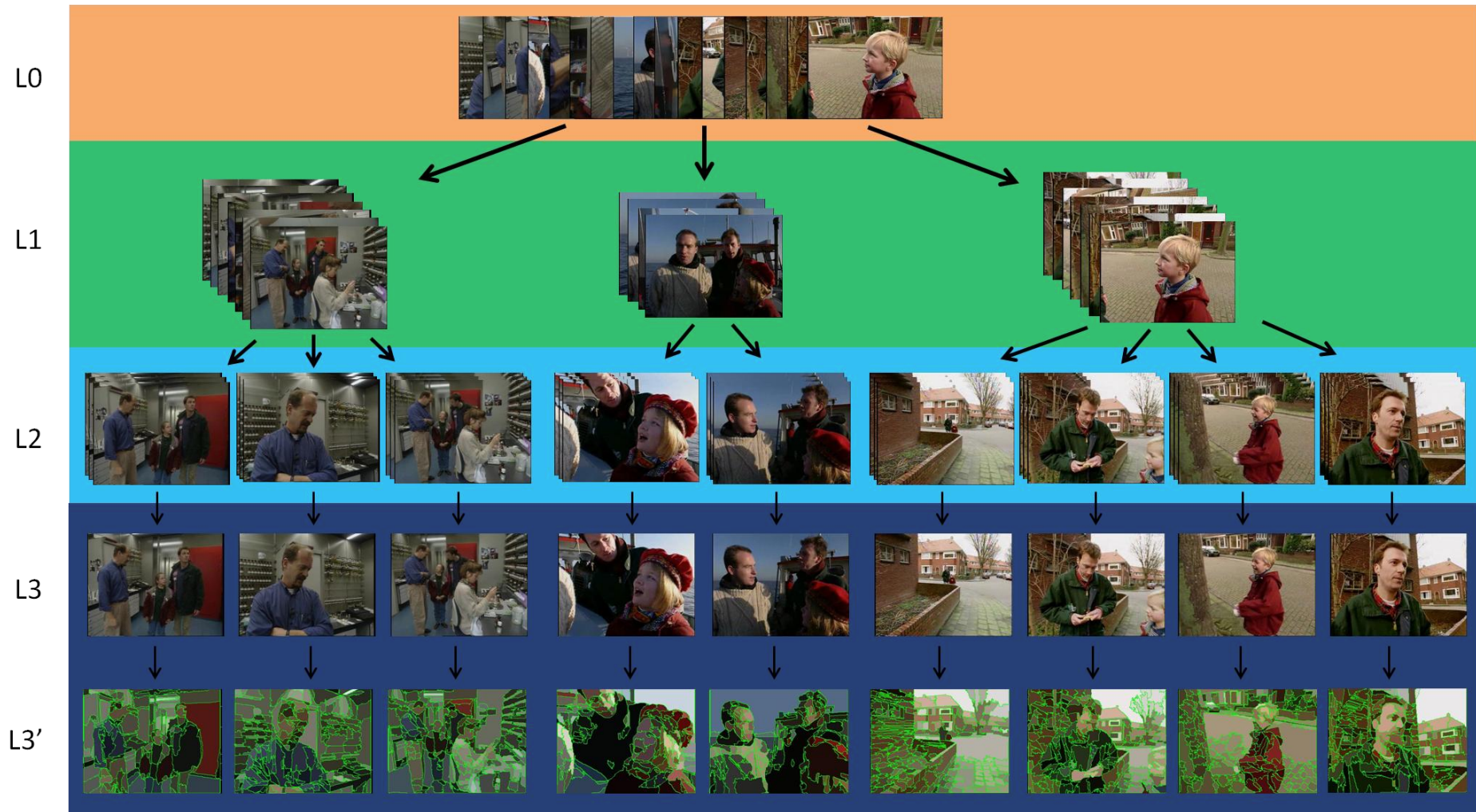
Figure 8.3. Hierarchical decomposition of a video (L0) in scenes (L1), shots (L2) and keyframes(L3). Level L3' concerns the regions from the keyframes, which are the entities used for video similarity in this case.
