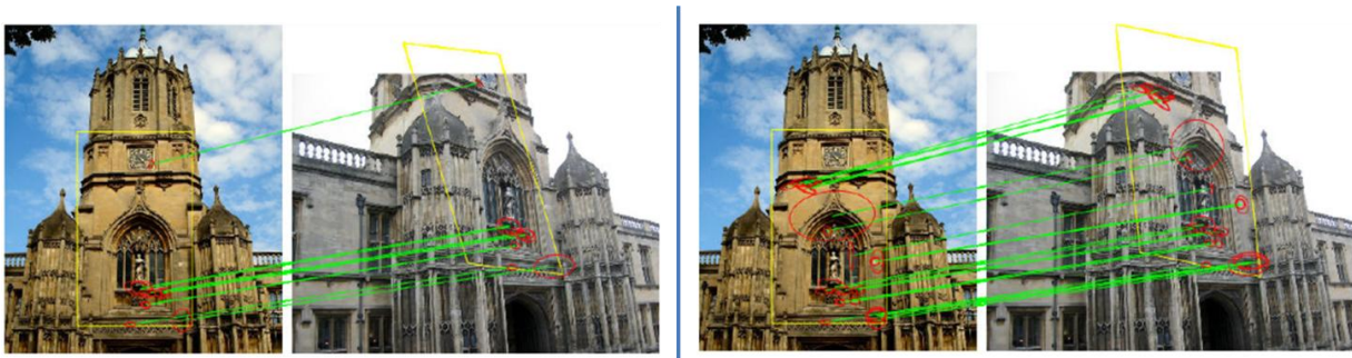
Figure 4.5. Comparison between SIFT and RootSIFT matching performances. On the left: SIFT with L2 distance - 10 matches. On the right: RootSIFT - 26 matches (illustration from [Arandjelovic 2012]).
