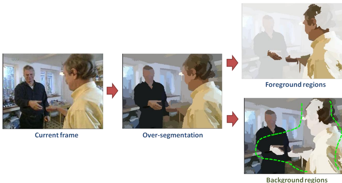
Figure 3.13. Background pseudo-scribbles extraction from a frame non-similar with the query frame illustrated in Figure 3.7. In this case we can notice that some of the filtered out regions are part of the queried object and they should be integrated back in the candidate object configuration. The color similarity of the border regions makes it possible to recover such regions and to reject other non-similar ones.
