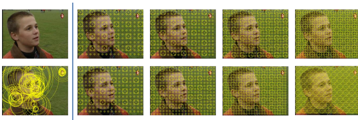
Figure 2.3. Dense sampling. In the first column we illustrate the original image and the regions detected by the Hessian-affine detector. In the rest of the columns dense sampling examples with various grid settings are illustrated. Notice how, for coarse grids many textured regions are missed, while for fine grids every patch of the image is sampled.
