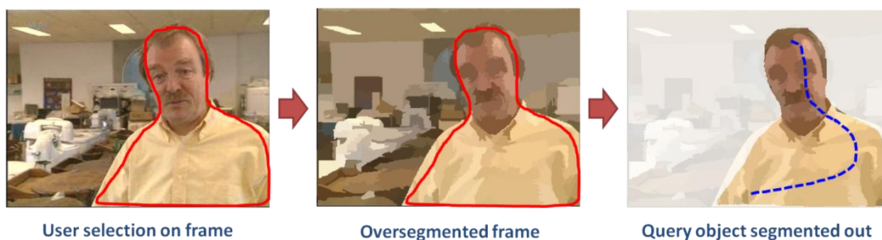
Figure 3.11. Query object extraction from user selection. After the regions composing the query model have been extracted, all these regions become foreground pseudo-scribbles (dashed blue-curve).
