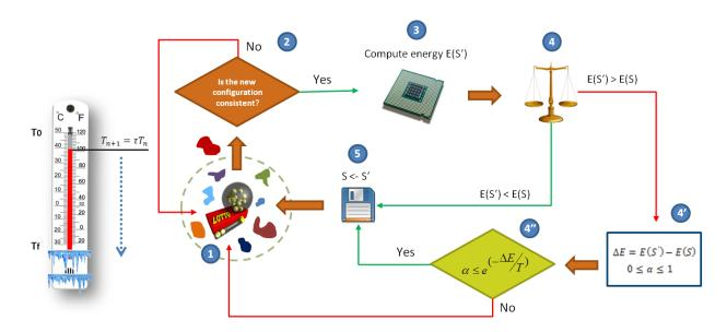
Figure 3.6. Overview on the Simulated Annealing implementation.
