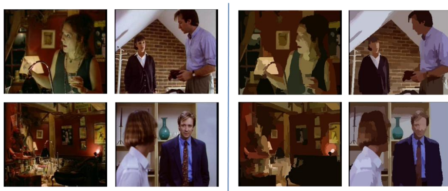
Figure 6.16. Video frames (left) and their segmentations (right). An average of 160 segmented regions provides in this case a “recognizable” image.
