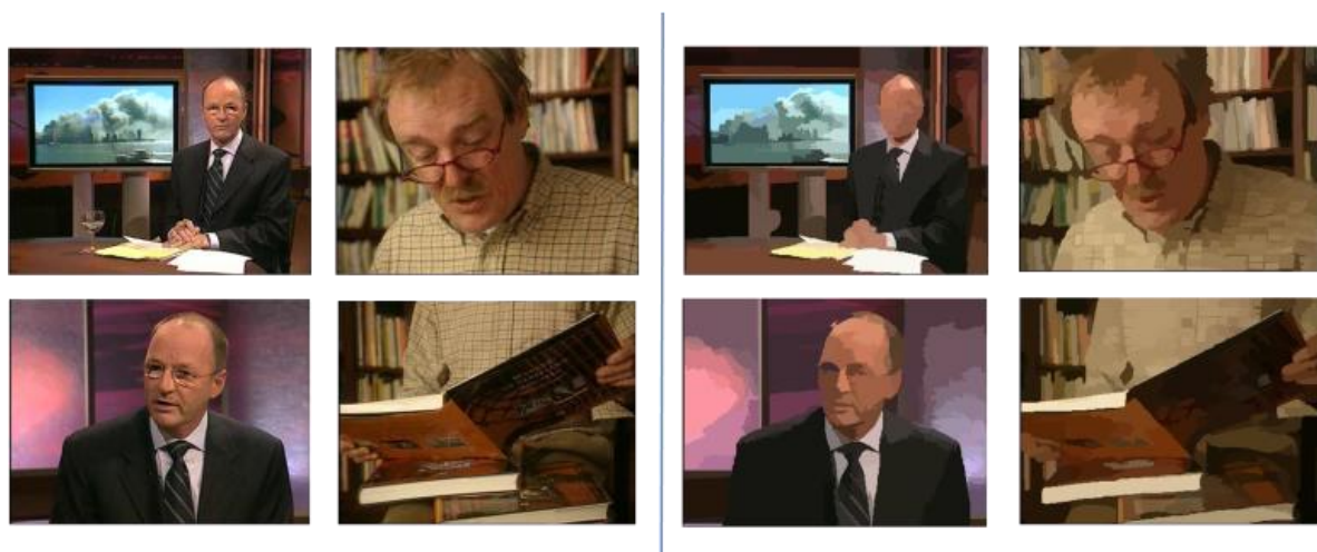
Figure 3.3. Video frames (left) and their MeanShift segmentations (right). A number of 200-300 segmented regions provides in this case a “recognizable” image. The regions are displayed with their corresponding Dominant Color.
