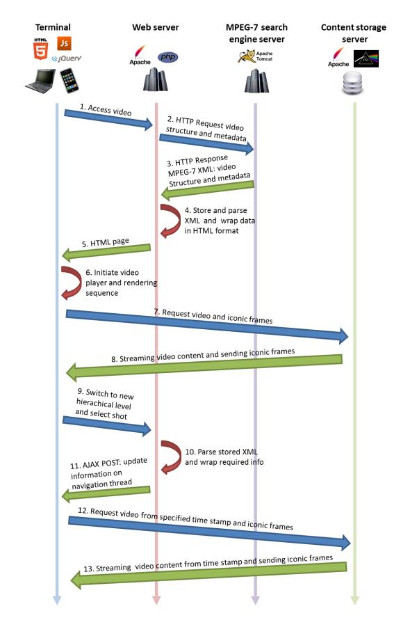
Figure 8.9. Timeline of events triggered when navigating in a video on the OVIDIUS platform.
