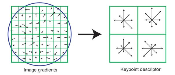
Figure 4.3. SIFT descriptor [Lowe 2004]. Image gradients within a patch (left) are accumulated into a coarse 4x4 spatial grid (right). In this example we show only a 2x2 grid. A histogram of gradient orientations is constructed in each grid cell. 8 orientation bins are used in each grid cell giving a descriptor with the dimension 128) 4x4x8 (illustration from [Lowe 2004]).
