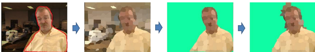
Figure 6.13. Query extension on SuperPixels 250. Regions under the scribble are added as a whole to the query object.
