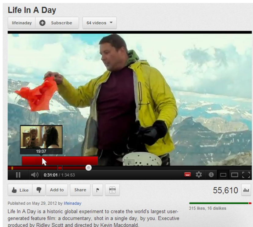
Figure 7.3. Advanced fine video preview and navigation using the video player time bar on YouTube [YouTube 2012]. A sliding window on the time bar grants finer access to the video segment underneath it. The second time bar is displayed above the main bar and mouse-over moves display key-frames from selected video time stamps.
