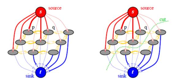
Figure 3.7. Graph construction in Greig *et. al.* Edge construction reflected by thickness. A graph G (left) and a cut on G (right).
