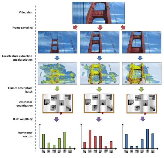
Figure 4.8. Frame-based BoW quantization.
