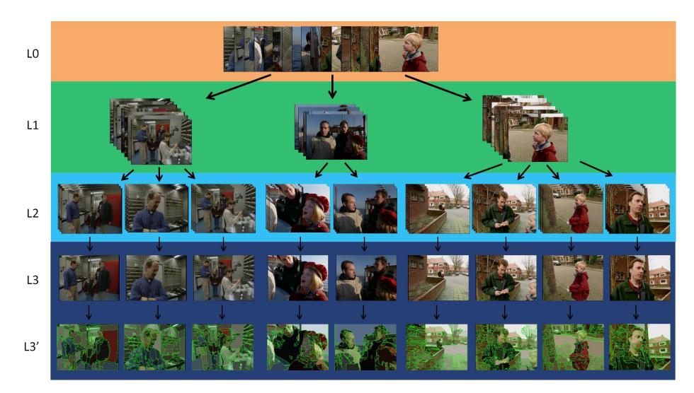
Figure 8.3. Hierarchical decomposition of a video (L0) in scenes (L1), shots (L2) and keyframes(L3). Level L3' concerns the regions from the keyframes, which are the entities used for video similarity in this case.
