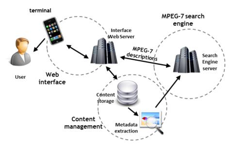
Figure 8.1. Overview of the architecture of the OVIDIUS platform.
