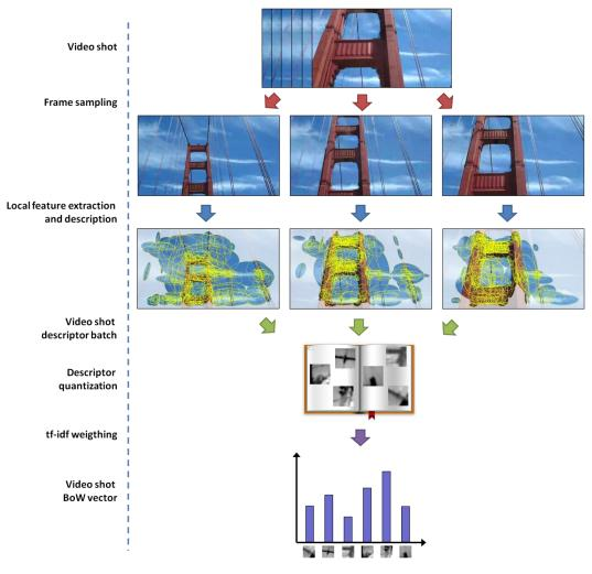
Figure 4.9. Shot based BoW quantization.
