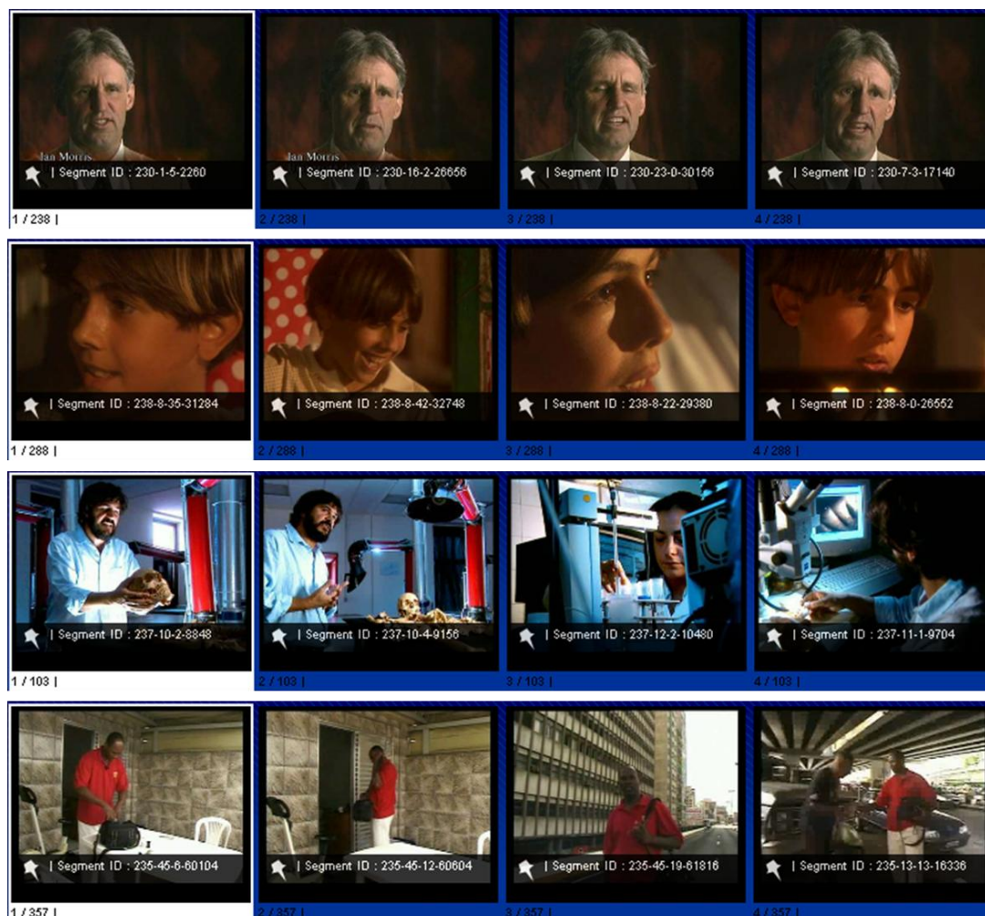
Figure 8.15. Search results based on MPEG-7 ColorStructure descriptor queries by example (first image of each row is the query image).
