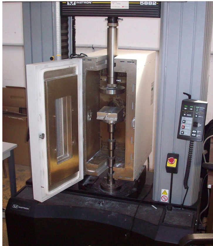
Figure A.2: Instron ® machine and its oven
