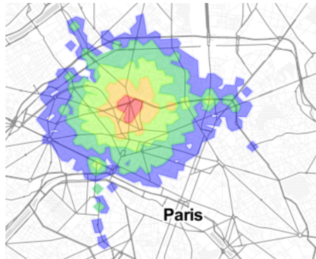
Figure 1.2: Isochrones: destinations reachable by using walking, public transportation, and rental bicycle after 3min (red), 6min (orange), 9min (light green), 12min (green), and 15min (violet) of travel time. Note that isochrone areas can be disconnected because stations of public transportation can often be reached faster than locations between stations. (Map: OpenStreetMap)
