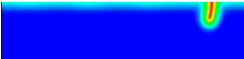
(c) Cracks longer then the damage band appear, thus necessarily a strong discontinuity in the evolution of the damage field  $\Theta = .6$ . height  $3.3\ell_0$ . On the left of the crack one observes 3 other beginning of localization which have not evolved into cracks
