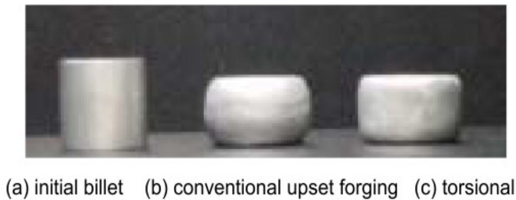
Figure 2-47. Photograph of experimental results ( h/d=1.0 , \gamma=30\% , \omega=0.264 ) (S. S. Youn et al., 2004) [44].
