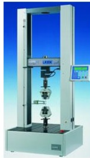
Figure 4-2. Lloyd machine LR30K.
