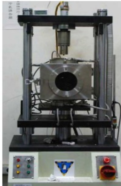
Figure 2-35. Ultrasonic hot upsetting experiment set up (J-C. Hung and C. Hung, 2005) [26].
