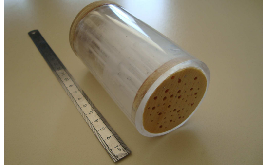
(b) Distribution bidisperse D_1 = 1025\mu m \pm 2,3\mu m et D_2 = 1895 \pm 1,5\mu m
