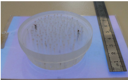
(d.1) Echantillon de distribution bimodale (\mu_1 = 350\mu\text{m}; \sigma_1 = 70\mu\text{m}) (\mu_2 = 630\mu\text{m}; \sigma_2 = 100\mu\text{m})
