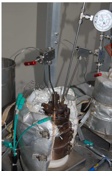
Figure 4.7: Picture of an autoclave used to prepare the Ox300°C stainless steel discs.
