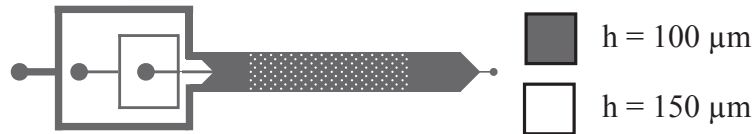
Figure 2.3: Chip geometry. The diameter of the anchor is 50 \mu\text{m} and is not to scale on this sketch.
