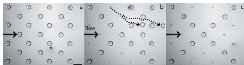
Fig. 2 Selectively extracting drops. (a) The array of holes ( d = 50 \mu\text{m} and p = 35 \mu\text{m} ) is initially filled with water drops. (b) The laser is focused on the water–oil interface, pushing the drops out of the anchor. (c) An X is patterned with the remaining droplets. Scale bar is 400 \mu\text{m} .
