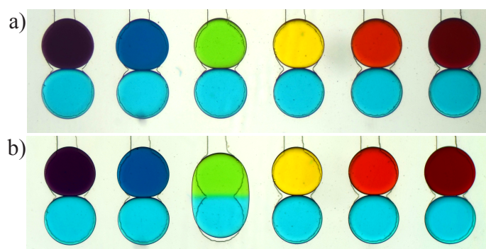
Figure 2.16: a) Array of six distinct pairs of droplets. b) A droplet pair has been merged on demand using a laser pulse.
