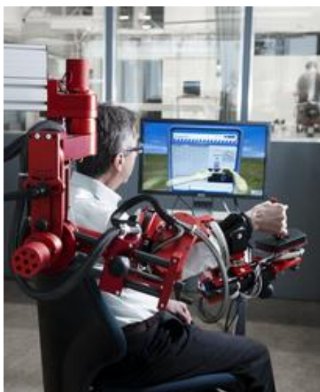
Figure 1.9: The ARMin exoskeleton for arm rehabilitation [Nef et al. 2009]
