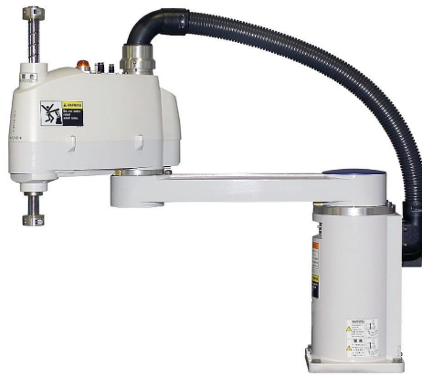
Figure 1.6: A typical serial robot (SCARA)
