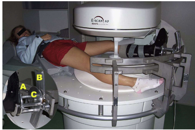
(b) MRI testbed for torsionally loaded knee. Inset shows loading apparatus for adjusting flexion-extension and ab/adduction rotations (A & B) along with internal-external rotation (C) [Hemmerich et al. 2009]
