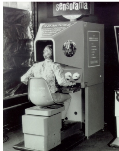
Figure 63: Sensorama Motion Picture Projector
