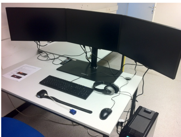
Figure 35: Experimental Setup - triple-screen display, instructions to read and the wireless pulse oximeter [source: author & Erik Geslin]
