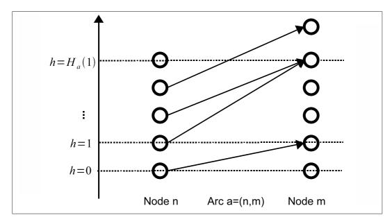
Figure 1.5: time-expansion of a dynamic network
