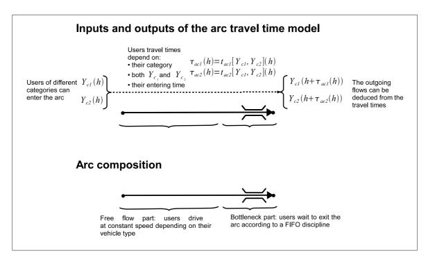
Figure 7.1: Arc travel time model principle
