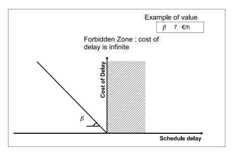
Figure 10.4: Schedule delay cost of the user category const. The value of  $\beta$  given here are just orders of magnitude. The value of  $\gamma$  is taken sufficiently high, that it is numerically close to infinity. The actual values used for the simulation are not given for confidentiality reasons.
