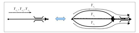
Figure 7.2: Multi-class dynamic loading principle A simple example for one arc with three vehicle classes. The flow represented by  $(Y_{c_1}, Y_{c_2}, Y_{c_3})$  is dispatched among three different routes on the new network.
