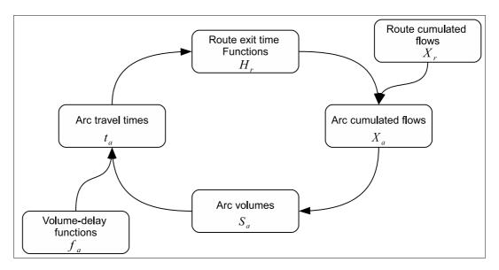
Figure 1.3: Relationship structure in the dynamic network loading problem adapted from (Leurent, 2003a)
