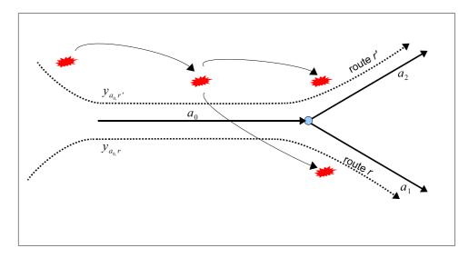
Figure D.7: Event Propagation in a DNLP. In this simple network, two routes are going through  $a_0$ . If an event occurs on route r', upstream arc  $a_0$ , it will cause an event on arc  $a_0$  and thus on all downstream arcs of route r
