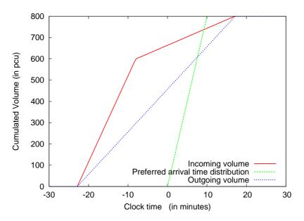
Figure 9.3: Results of the user coordination algorithm on one arc after 20 iterations
