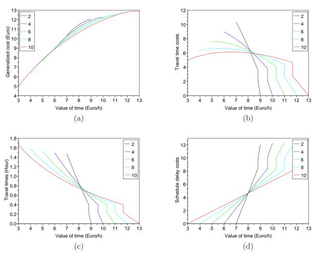
Figure 6.12: For different values of the spread in the high toll case: (a) generalized costs for different values of the spread in the high toll case, (b) travel costs, (c) travel times, and (d) schedule delay costs
