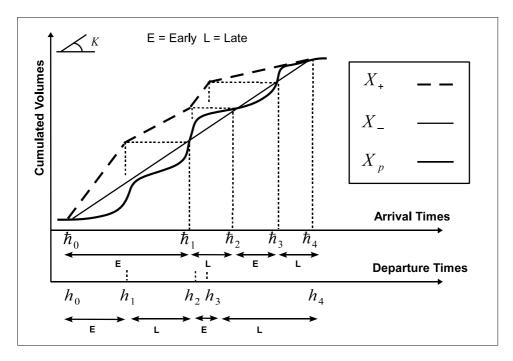
Figure 5.2: Critical times at arrival and at departure
