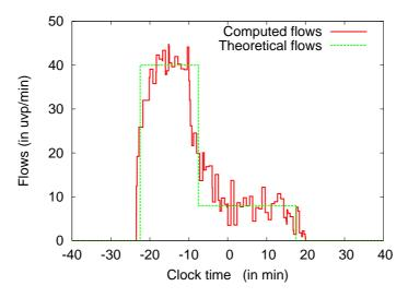
Figure 8.10: Numerical results of the UE computation algorithm with a V-shaped schedule delay cost function - flows
