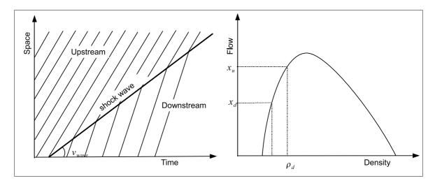
Figure 1.1: Shock waves with the LWR model: flow density relationship (right) and time space diagram (left)
