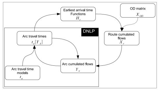
Figure 2.1: Relationship structure in the dynamic Wardrop assignment (Figure of the top adapted from (Leurent, 2003b))
