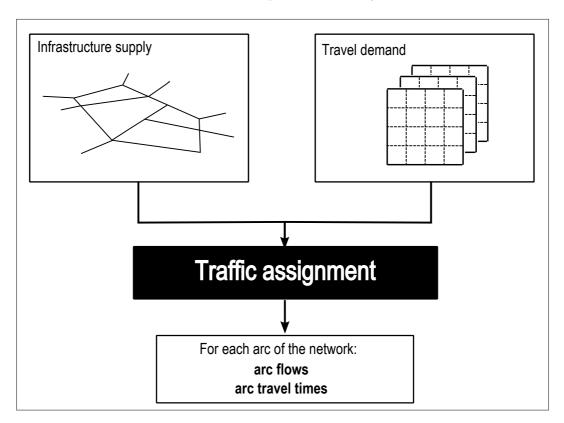
Figure 1: General framework of a traffic assignment procedure
