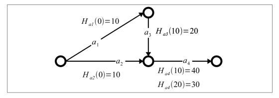
Figure 1.4: Route inconsistency in non-FIFO networks
