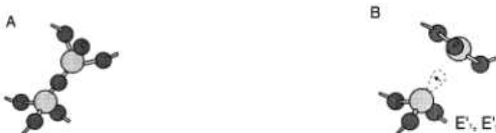
Figure III-15. A) fragment of perfect lattice; B) the "classic" model of E' 1 center in \alpha -quartz or E' v center in silica, from L. Skuja's review [21]
