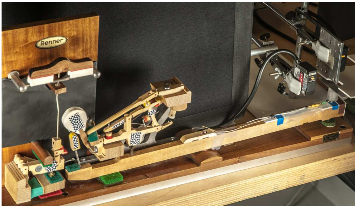
Figure 3.16 – Photography of the piano action showing the tracking patterns, the accelerometer, the two lasers, the force sensor and the piston.
