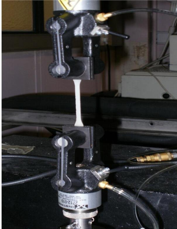
*Figure 2-6: Tensile machine*
