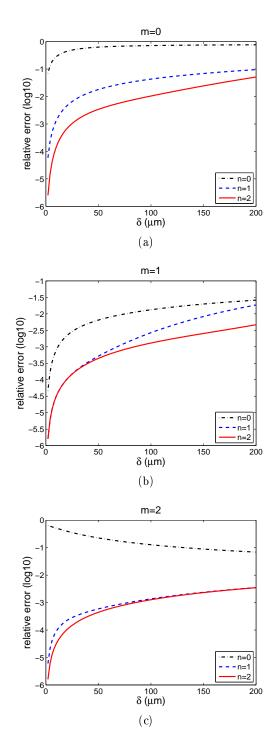
Figure 3.3:  $L^2_{1/2}$ -norm relative errors of asymptotic models with  $\mathcal{Z}_{m,n}$  transmission conditions. Comparison between different expansion order n, rescaling parameter m fixed.
