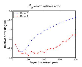
Figure 4.2: Relative error of the asymptotic models using  $\mathcal{Z}_{1,n}$  transmission conditions, n = 0, 1.
