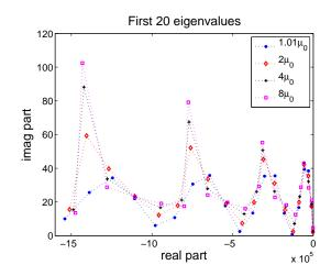
Figure 1.7: First 20 eigenvalues for different tube permeabilities.
