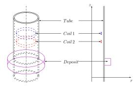
Figure 1.1: Three- and two-dimensional geometric representations of a steam generator tube covered with deposits and a probe consisting of two coils.
