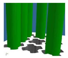
(a) SG tubes and a broached quatrefoil support plate.
