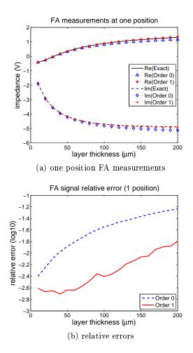
Figure 4.3: Approximation of impedance measurements using asymptotic models with  $Z_{1,n}$ , n = 0, 1.
