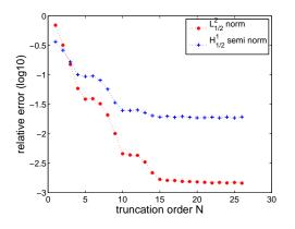
Figure 1.4: Relative errors for eddy current simulations using DtN maps with different truncation orders N.
