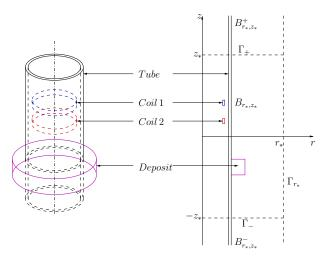
Figure 2.1: 3-D and 2-D geometrical representations of a SG tube covered with deposits and a probe consisting of two coils.
