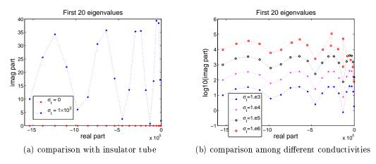
Figure 1.6: First 20 eigenvalues for different tube conductivities.
