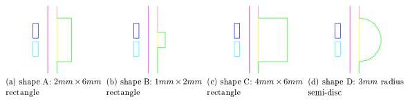
Figure 1.8: Different deposit shapes.
