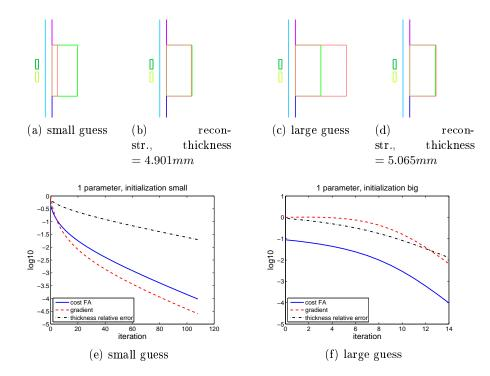
Figure 2.4: Results of thickness reconstruction of a rectangular non-magnetic deposit.
