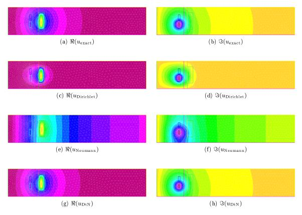
Figure 1.5: Real and imaginary parts of u fields on cut-off domain using different boundary conditions. DtN maps of truncation order N = 20.
