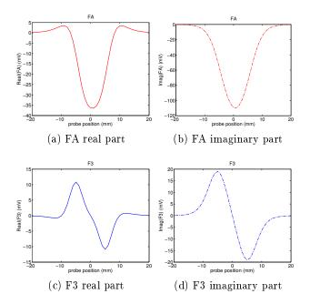
Figure 2.2: ECT signals of a rectangular deposit.
