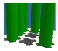
Figure 5.1: SG tubes maintained by a broached quatrefoil support plate.
