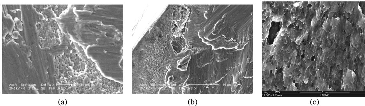
Fig. III-18 SEM views of fracture surfaces of broken notched specimens (a) steel  $\beta = 0^\circ$  (b) steel  $\beta = 55^\circ$  (c) alu-1  $\beta = 0^\circ$  (d) alu-1  $\beta = 55^\circ$  (e) steel in-situ torsion test.
