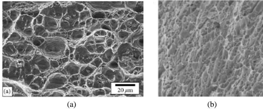
Fig. 0-9 Ductile fracture surfaces of (a) an aluminum 2024-T351 sheet (Bron et al. [8]) and (b) a Weldox 420 tubular specimen with torsion-dominant loading (Barsoum and Faleskog [6])
