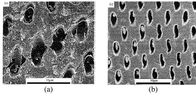
Fig. 0-12 Coalescence by (a) internal necking and (b) void sheeting in copper sheets (Weck et al. [17])
