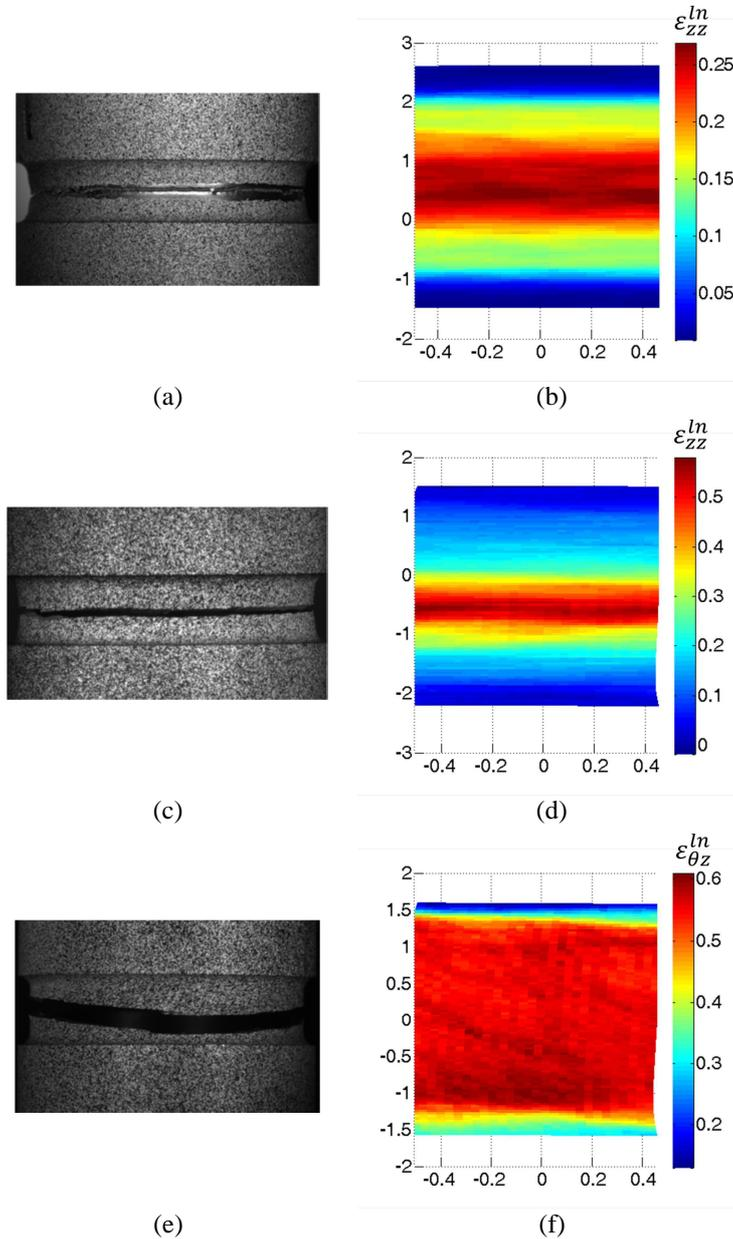
Fig. I-7 Photographs of the fractured specimens and measured surface strain fields at the onset of fracture. (a)-(b)  $\beta = 90^\circ$ , (c)-(d)  $\beta = 55^\circ$ , (e)-(f)  $\beta = 0^\circ$ .
