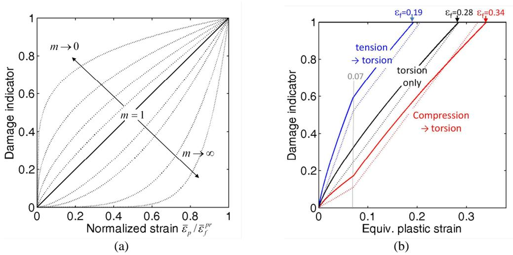
Fig. II-12 Non-linear damage accumulation law: (a) Effect of the exponent  $m$  including the special case of linear damage accumulation for  $m=1$ , (b) Evolution of damage in a torsion experiment after pre-loading under tension (blue) and compression (red), as well as for proportional loading (black); the dashed lines show the predictions for linear damage accumulation ( $m=1$ ), the solid lines depict the results for non-linear damage accumulation ( $m=0.8$ ).
