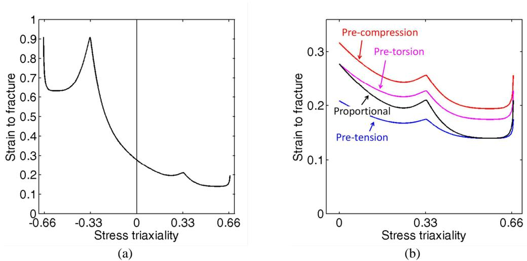
Fig. II-11 (a) Hosford-Coulomb fracture envelope for proportional plane stress loading; (b) Fracture envelope for  $\eta \geq 0$  after pre-loading up to  $\bar{\epsilon}_p = 0.07$  under uniaxial compression ( $\eta = -0.33$ , red curve), uniaxial tension ( $\eta = 0.33$ , blue) and transverse plane strain tension ( $\eta = 0.58$ , magenta). (a=1.21, b=0.21, c=0.076, m=0.71)
