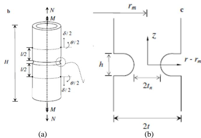
Fig. 0-5 Tension-torsion specimen used by Barsoum and Faleskog [6]
