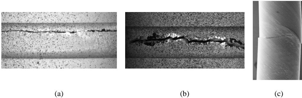
Fig. III-5 Circumferential view of broken notched specimens for notched specimens of alu-1 (a)  $\beta=0^\circ$  and (b)  $55^\circ$ . (c) View of broken specimens from the torsion in-situ tests on alu-2.
