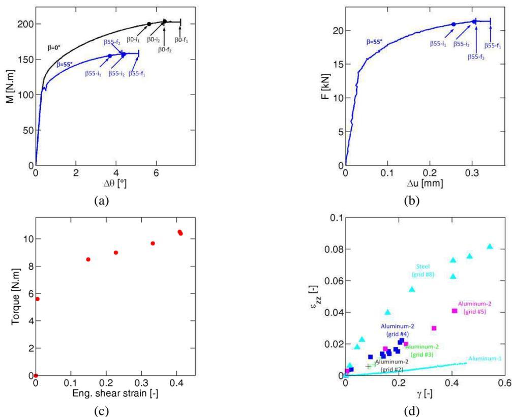
Fig. III-4 Load VS displacement curves (a)  $M$  VS  $\Delta\theta$  and (b)  $F$  VS  $\Delta u$  for interrupted tests and tests to fracture on alu-1 notched tubular specimens (c)  $M$  VS  $\gamma$  for the in-situ torsion test on alu-2 (d) Evolution of the engineering axial strain versus the engineering shear strain measured during in-situ tests.
