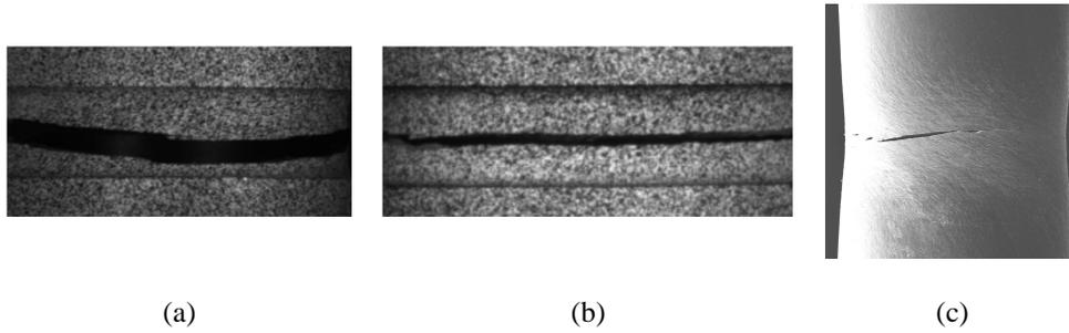
Fig. III-16 Circumferential view of broken notched specimens for steel notched specimens: (a)  $\beta=0^\circ$  and (c)  $55^\circ$ ; (c) View of broken specimens from the torsion in-situ tests on the steel cylindrical I specimen.
