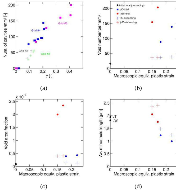
Fig. III-11 (a) Evolution of the void number per surface unit for the in-situ torsion test on alu-2. For the interrupted tests on notched specimens on alu-1, evolution of the (b) number per surface unit (c) area fraction (d) average minor axis.
