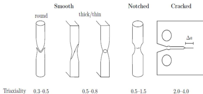
Fig. 0-3 Common specimens geometry (Benzerga and Leblond, [2])
