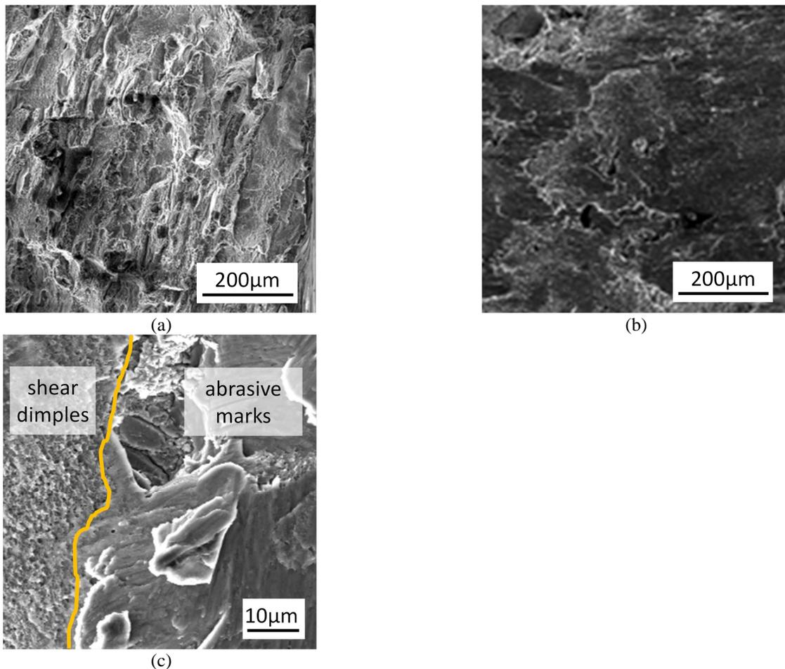
Fig. II-6 SEM view of fracture surfaces: (a) dimpled surface as observed for  $\beta=90^\circ$ , (b) abrasive marks as observed for  $\beta=55^\circ$ , (c) shear dimples and abrasive marks observed for  $\beta=0^\circ$ .
