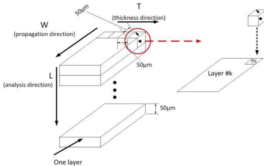
Fig. IV-2 Computation of the void volume fraction field.
