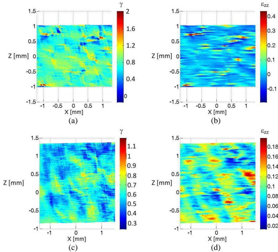
Fig. III-6 Interrupted tests on alu-1. Surface strain fields measured by 3DIC just before fracture for  $\beta 0\text{-i}_2$  (a) engineering shear and (b) axial strain, and for  $\beta 55\text{-i}_2$  (c) engineering shear and (d) axial strain
