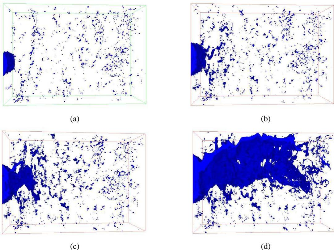
Fig. IV-6 3D view of thresholded sub-volumes ( $T \times W \times L = 770 \times 1335 \times 940\mu\text{m}^3$ ) for (a)  $\delta_5= 0\mu\text{m}$  (b)  $\delta_5= 27.6\mu\text{m}$  (c)  $\delta_5= 42.5\mu\text{m}$  (d)  $\delta_5= 77.4\mu\text{m}$
