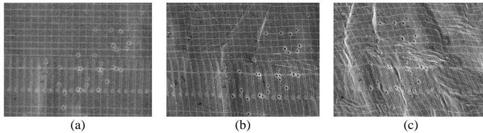
Fig. III-21 Evolution of preexisting cavities during the in-situ torsion test on the steel (a)  $\gamma=0$  (b)  $\gamma=0.105$  (c)  $\gamma=0.372$
