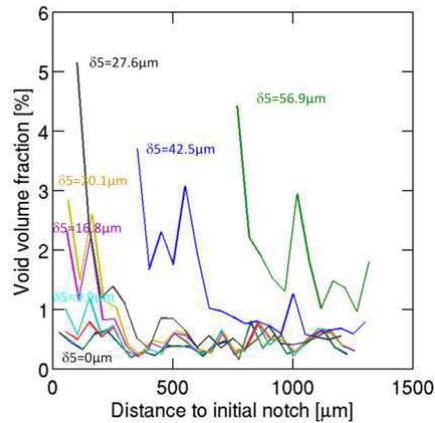
Fig. IV-9 Evolution of average void volume fraction versus the distance to the initial crack front
