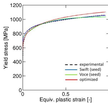
Fig. I-9 Identification of the isotropic hardening law.
