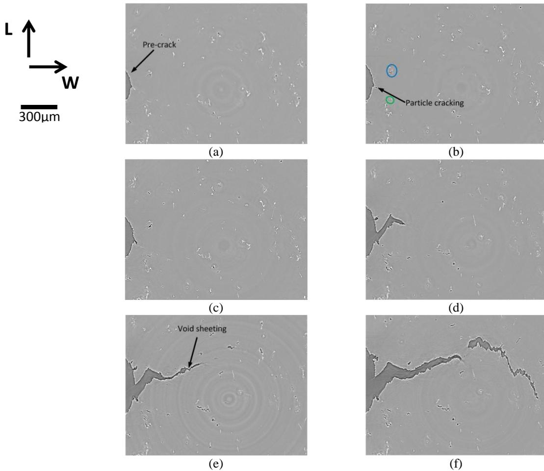
Fig. IV-3 2-D sections in the LW plane at mid-thickness of the specimen for  $\delta_5 =$  (a)  $0\mu\text{m}$  (b)  $9.8\mu\text{m}$  (c)  $16.8\mu\text{m}$  (d)  $42.5\mu\text{m}$  (e)  $56.9\mu\text{m}$  (f)  $77.4\mu\text{m}$
