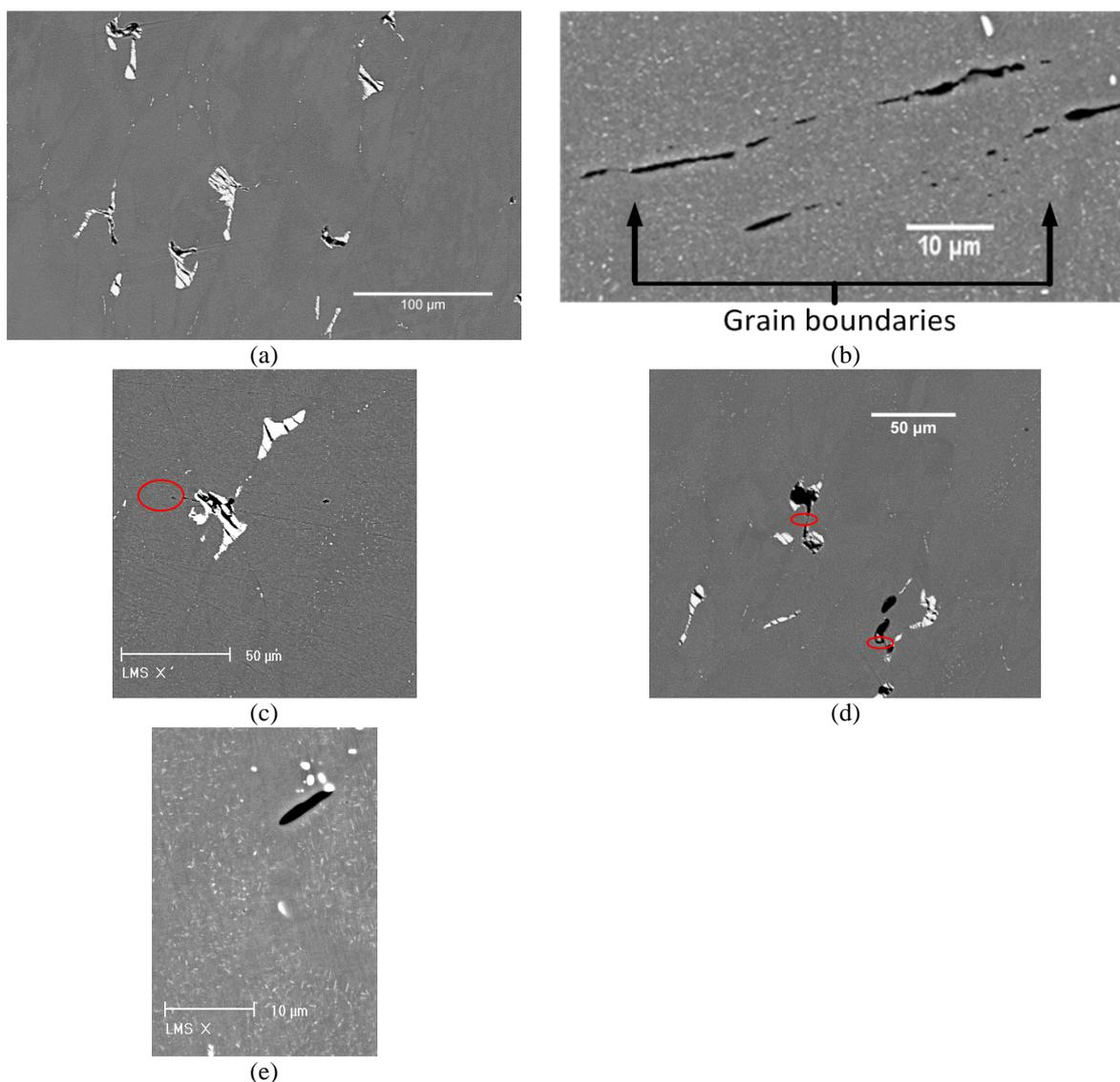
Fig. III-10 SEM micrographs from interrupted tests on notched tubular specimens of alu-1 (a)  $\beta_{55-i_1}$  (b)  $\beta_{0-i_2}$  near the crack (c)  $\beta_{0-i_2}$  very coarse particle fracture near a grain boundary and nucleation of micro-voids (d)  $\beta_{0-i_2}$  a very elongated void (e)  $\beta_{55-i_2}$  void sheeting coalescence
