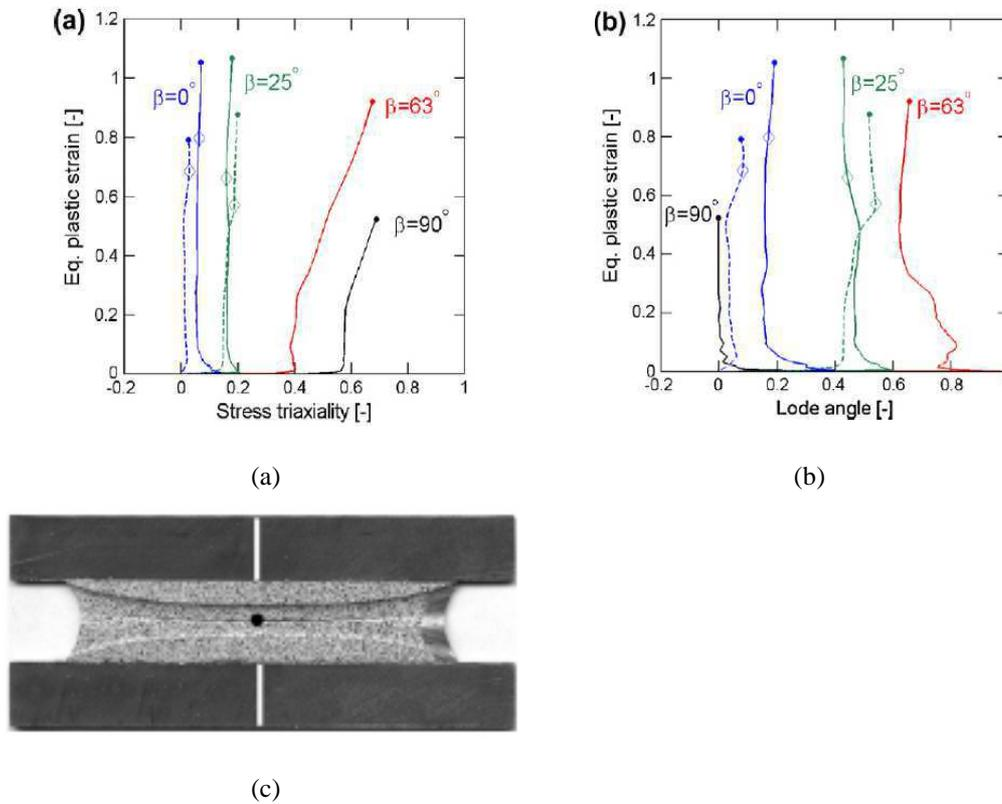
Fig. 0-8 (a) and (b) loading paths to fracture in the spaces  $\{\bar{\eta}, \bar{\varepsilon}_p\}$  and  $\{\bar{\theta}, \bar{\varepsilon}_p\}$  (c) optimized butterfly specimen in combined shear and tension (Dunand and Mohr [7])
