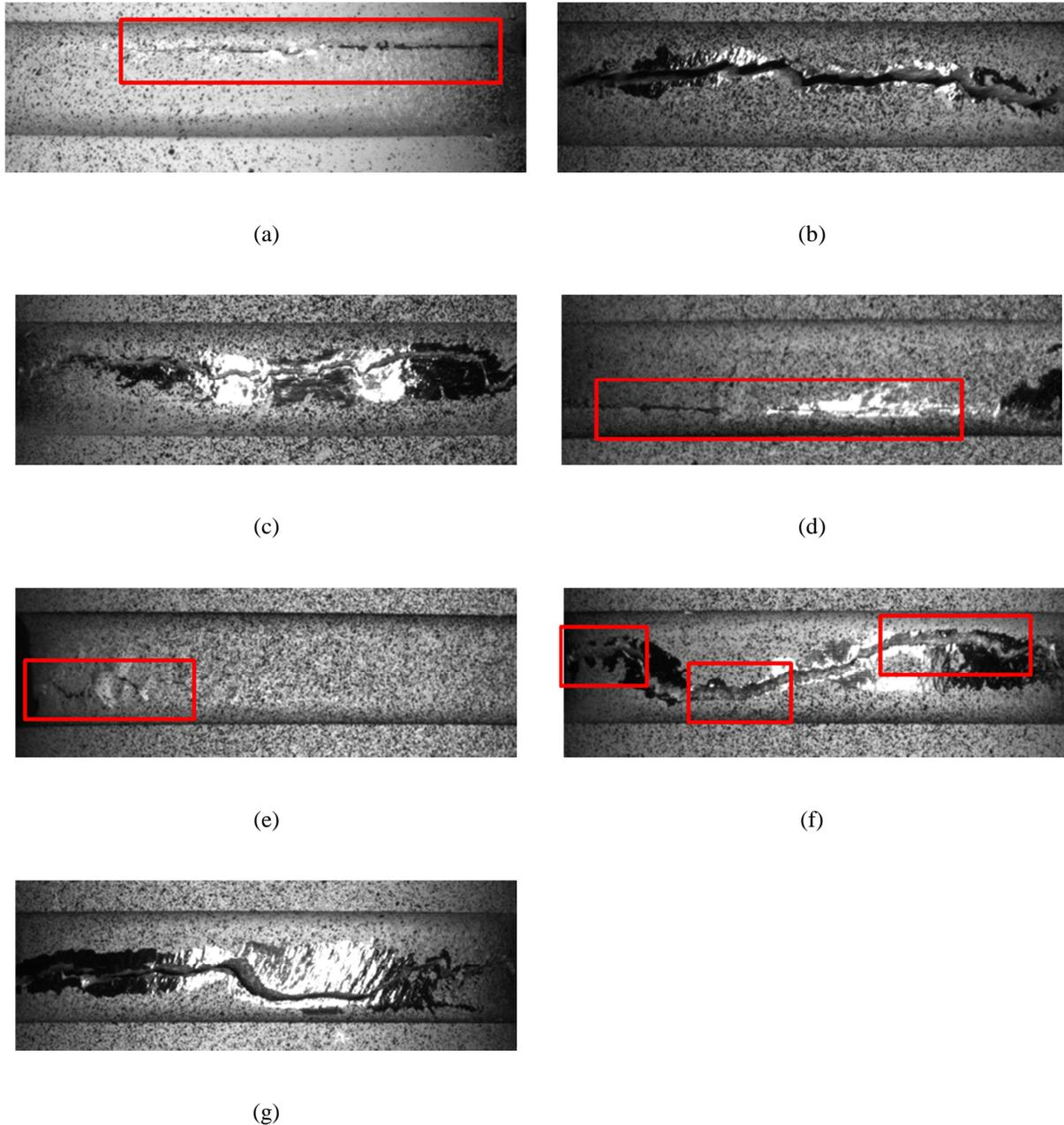
Fig. II-5 Pictures of a few broken specimens (a) proportional  $\beta=0^\circ$  (b) proportional  $\beta=55^\circ$  (c) proportional  $\beta=90^\circ$  (d)  $\beta=0^\circ$  with pre-compression (e)  $\beta=55^\circ$  with pre-tension (f)  $\beta=90^\circ$  with pre-torsion (g)  $\beta=55^\circ$  with pre-torsion.
