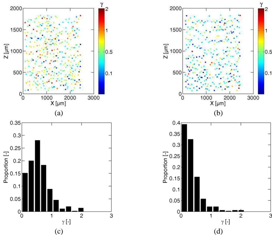
Fig. III-7 Alu-1. Engineering shear strain obtained from grain morphological rotation for (a)  $\beta_0$ - $i_1$  and (b)  $\beta_{55}$ - $i_1$ . Local shear distribution for (c)  $\beta_0$ - $i_1$  and (d)  $\beta_{55}$ - $i_1$ .
