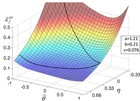
Fig. II-10 Hosford-Coulomb fracture envelope identified for aluminum 2024-T351 ( $a=1.21$ ,  $b=0.21$ ,  $c=0.076$ ,  $m=0.71$ )
