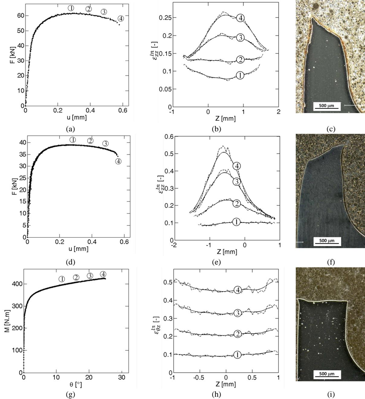
Fig. I-8 Evolution of the surface strains throughout loading: (a)-(c)  $\beta = 90^\circ$ , (d)-(f)  $\beta = 55^\circ$ , and (g)-(i)  $\beta = 0^\circ$ . The solid (dashed) lines in the central plots correspond to the strains obtained from the displacement measurements with (without) averaging over a 200  $\mu\text{m}$  period. The rightmost column shows longitudinal cuts through the fractured specimens.
