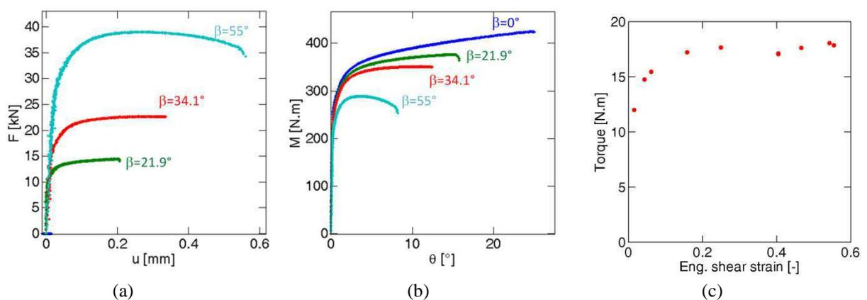
Fig. III-15 Load VS displacement curves (a)  $F$  VS  $\Delta u$  and (b)  $M$  VS  $\Delta \theta$  for interrupted tests and tests to fracture on steel notched tubular specimens; (c)  $M$  VS  $\Delta \theta$  for the in-situ torsion test on steel.
