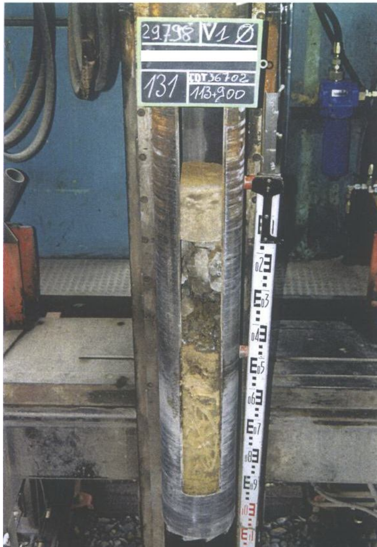
Fig. 10: Core sample from typical ancient railway sub-structure
