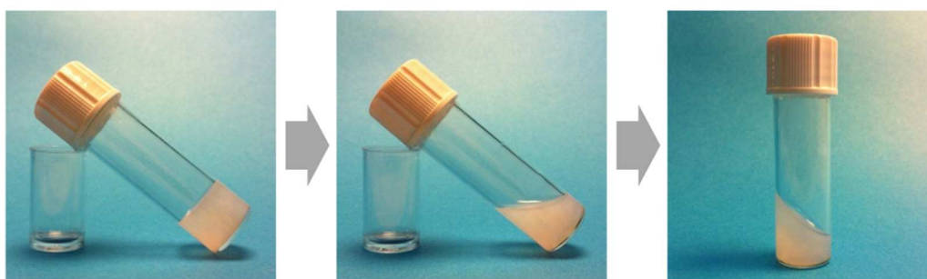
Figure 3.16. Photographs of a phase tuned \text{LaPO}_4 nanorod suspension in ethylene glycol showing a dramatic thixotropic behavior, left – original gel state, middle – sol state after stirring, right – returned gel state after setting the sol inclined.
