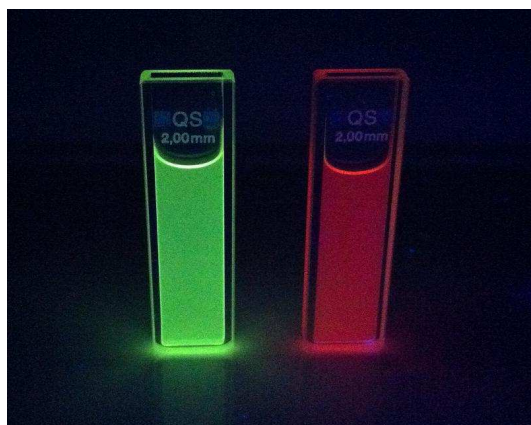
Figure 4.1. Photograph of aqueous suspensions of luminescent Ce 0.45 Tb 0.15 La 0.4 PO 4 (green emission) and Eu 0.05 La 0.95 PO 4 (red emission) nanorods under UV lamp irradiation ( \lambda_{\text{exc}} = 260\text{nm} ).
