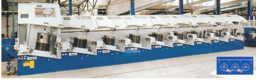
Fig. 1.5: Multi-pass wire drawing machine (Ugitech).
