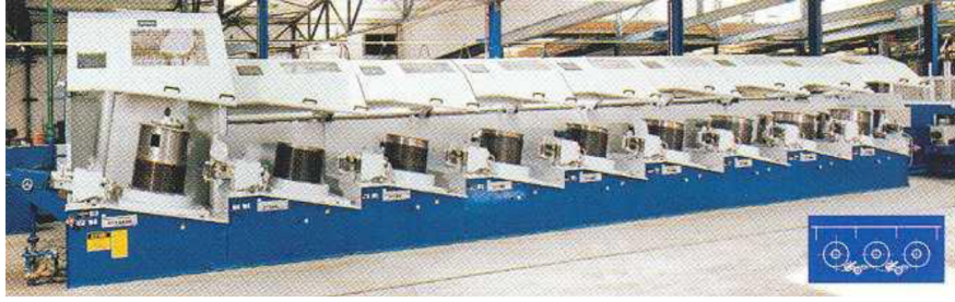
Fig. 1.5: Multi-pass wire drawing machine (Ugitech).
