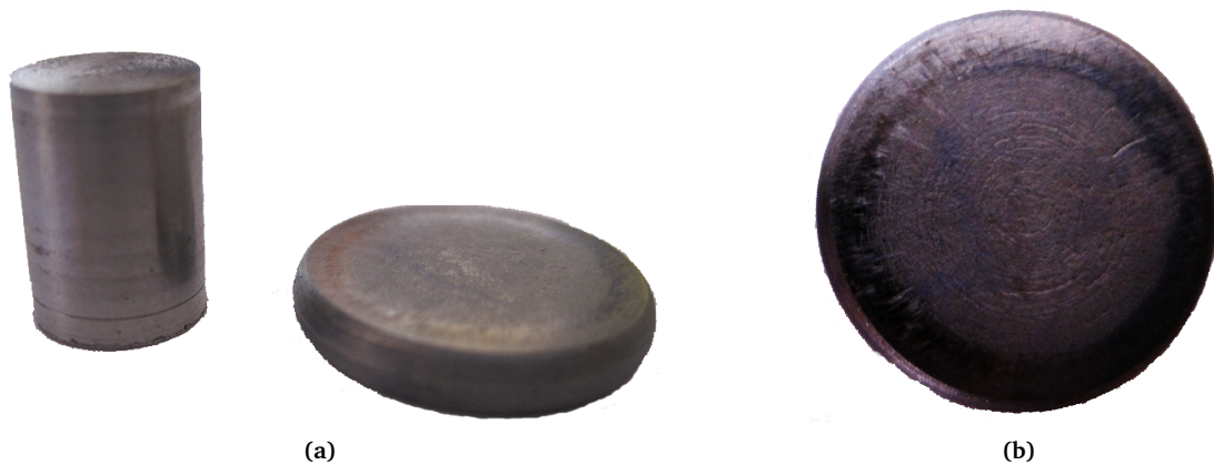
Fig. 2.7: (a) The compression specimens before and after deformation, and (b) the end of the compression specimen. The darker central region was the original end. The lighter region outside was originally part of the cylindrical wall that folded up due to severe barreling.
