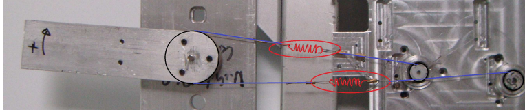
Figure 15.14: Experimental setup used for the verification of the backstepping controller
