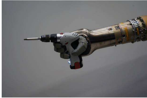
Figure 1.10: Dexhand a space qualifiable hand from DLR
