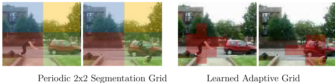
Figure 5-4: Illustration des fixed versus task-specific grids. Task-specific grid coarsely follows the action through time.
