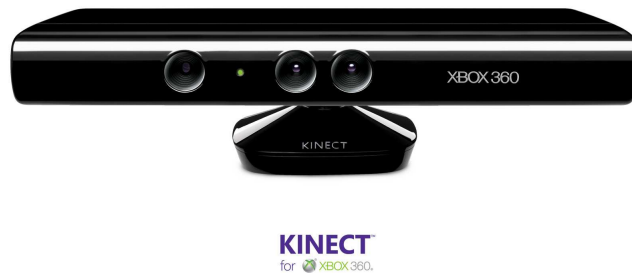
Figure 4.20: The Kinect device, released by Microsoft in November 2010. It provides RGBD data, which enables motion estimation techniques based on combined processing of image and depth, as presented in this part.
