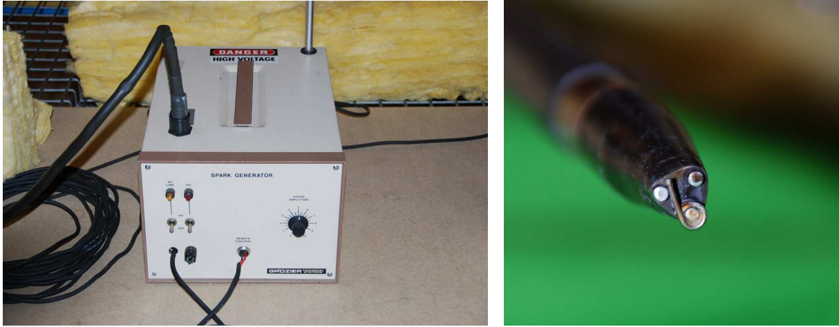
Figure 7.2: Spark source Grozier GTS 51. The generator charges a capacitance, which can then be discharged across close electrodes. The electrodes are located at the end of a wand attached to the generator. Left: spark generator itself. Right: zoom on the electrodes, located at the end of the wand. Spacing between the electrodes is of the order of 3 mm.
