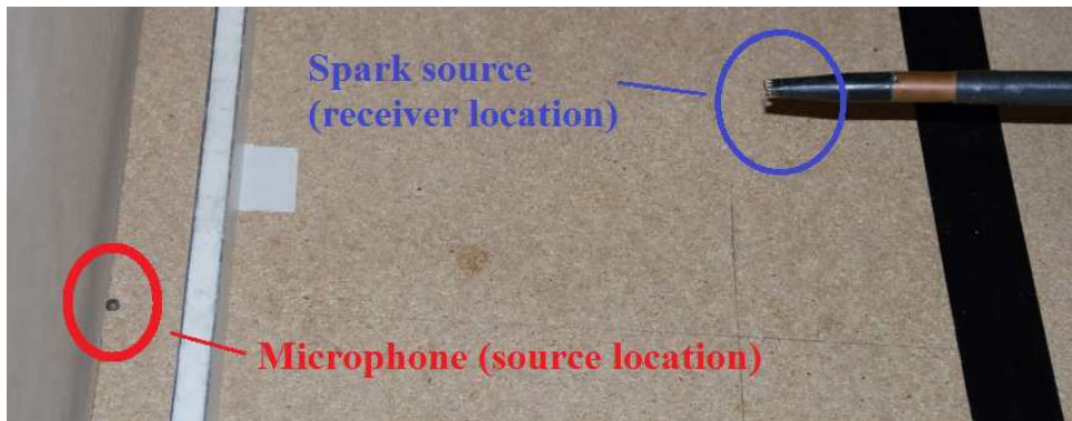
Figure 7.7: Spark source and microphone positions in the scale model measurement. Using reciprocity, source and receiver positions have been exchanged, so that the B&K 1/4" microphone lies at the ground level and represents the actual source, whereas the spark is generated at the actual receiver position, behind the barrier.
