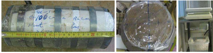
Figure 2-24 Water content protection and volume measurement
