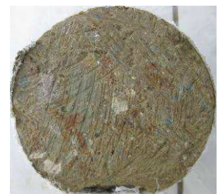
(c) High stiffness at 3.8 m (1132 MPa)
