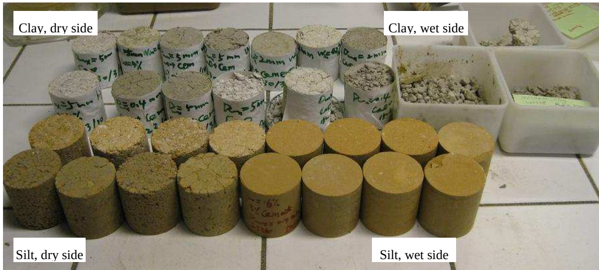
Figure 2-17 Some specimens after water content measurement, during water loss test
