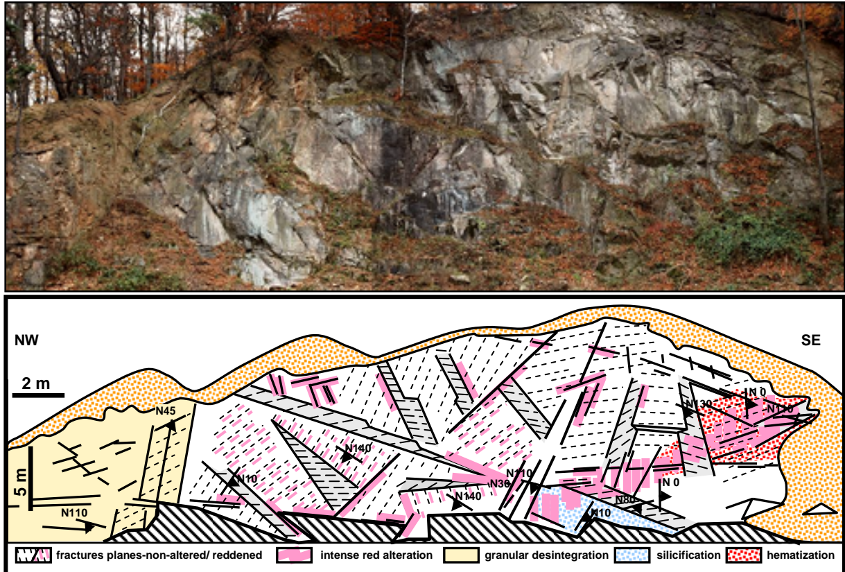
Figure 8 – Picture and sketch of the red alteration that follows the fractures in the Laski quarry. The highly fractured zones, in the SE of the quarry are the most reddened. A direct relation exists between fractures frequency and the intensity of the alteration.
