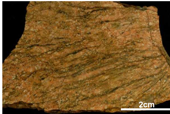
Figure 20 – Reddening within the Haniak gneiss from the Kopciowa Mountain. The pinkish bands are quartzo-feldspathic while dark bands contain biotites.
