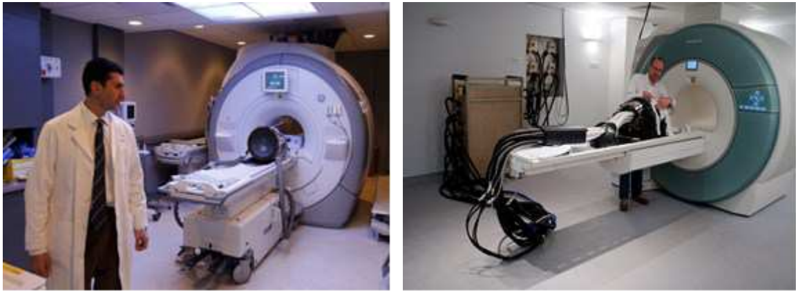
Figure 2.11: Systems for transcranial treatments Insightec (Left, 660 kHz) and SuperSonic Imagine (right, 1 MHz).
