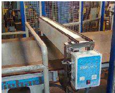
Figure 1.24: The 'Meplaca' measurement system [Indwitech website]
