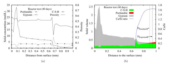
Figure 7.20: After 40 days of test in simulation reactor: (a) Solid concentration and porosity; (b) Solid volume and Ca/Si ratio of C-S-H. (H<sub>2</sub>S level = 400 ppm)
