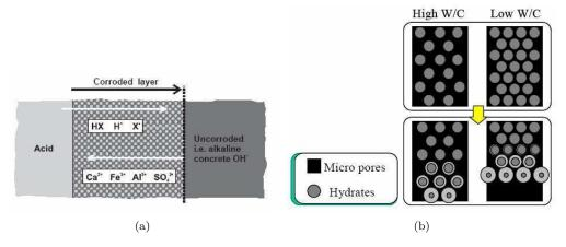
Figure 4.3: Schematics of the microstructure of cementitous materials with uncompressed gypsum inclusion: (a) Through-solution mechanism (Beddoe and Dorner, 2005); (b) Deposition in pores mechanism (Kawai et al., 2005)
