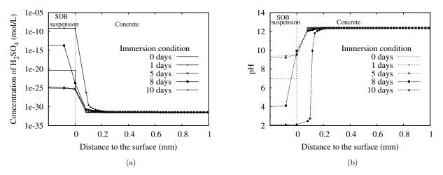
Figure 7.12: The calculated  $H_2SO_4$  and pH evolution profiles in SOB suspension and concrete from 0 days to 10 days: (a)  $H_2SO_4$  concentration; (b) pH value.
