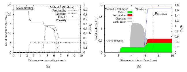
Figure 6.12: After 90 days of immersion: (a) Solid concentration and porosity; (b) Solid volume and Ca/Si ratio of C-S-H .  $D_{Simulation}$  and  $D_{Experiment}$  represent the degradation depth of the sample in simulation and experiment individually. (Method 2, pH=1)
