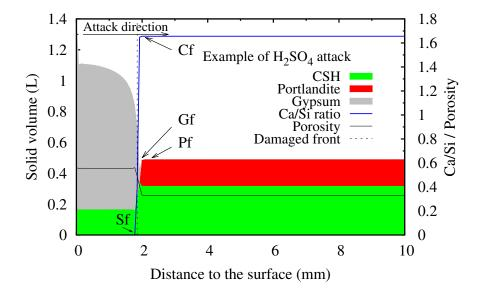
Figure 5.3: Solid profiles after 15 days immersion
