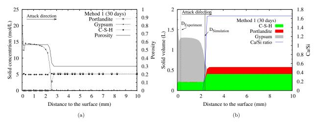
Figure 6.4: After 30 days of immersion: (a) Solid concentration and porosity; (b) Solid volume and Ca/Si ratio of C-S-H .  $D_{Simulation}$  and  $D_{Experiment}$  represent the degradation depth of the sample in simulation and experiment individually. (Method 1, pH = 1)
