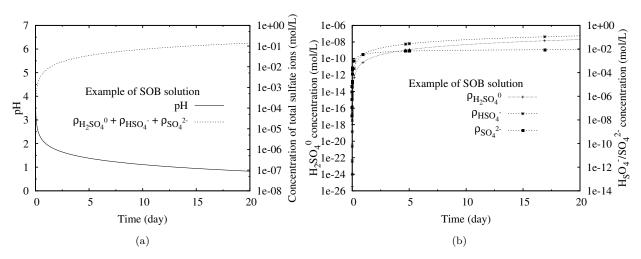
Figure 5.10: In SOB solution without cement paste: (a)  $p{\rm H}$  and the concentration of total sulfate ions ; (b) Concentration of  ${\rm H_2SO_4}^0$ ,  ${\rm HSO_4}^-$  and  ${\rm SO_4}^{2-}$
