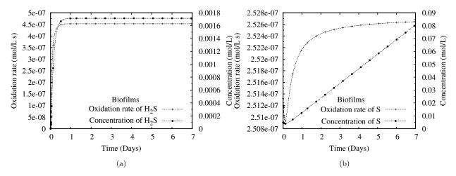
Figure 7.18: The oxidation of  $H_2S$  and S versus their concentration in the biofilms: (a) Aqueous  $H_2S$ ; (b) Element S. ( $H_2S$  level = 400 ppm)
