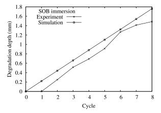
Figure 7.15: The predicted and measured corrosion depth.
