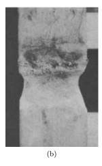
Figure 7.16: Mortar specimens exposed to H<sub>2</sub>S gas: (a) Water; (b) Sewage. (Mori et al., 1992).
