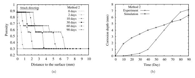
Figure 6.15: The predicted evolution of porosity and corrosion depth profiles from 0 days to 90 days: (a) Porosity; (b) Corrosion depth. (Method 2, pH = 1)
