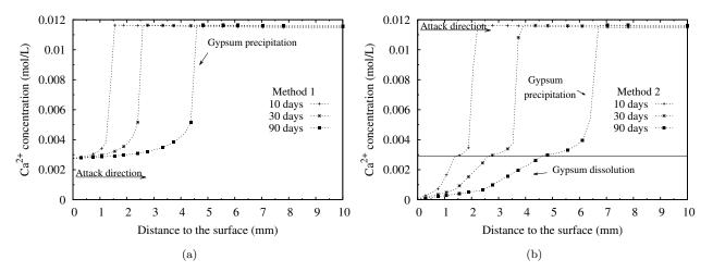
Figure 6.13: The calculated  $Ca^{2+}$  concentration profiles during immersion: (a) Method 1; (b) Method 2. (pH = 1)
