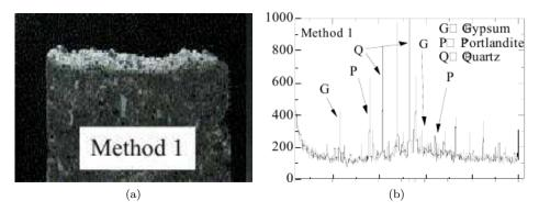
Figure 6.1: After 90 days immersion test: (a) Observation of deterioration of sample; (b) XRD patterns of surface area of sample. (Method 1, pH = 1) (Kawai et al., 2005)
