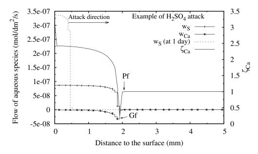
Figure 5.7: Flow of calcium and sulfur and  $\zeta_{\rm Ca}$  after 15 days immersion
