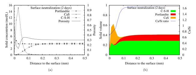
Figure 7.7: After 2 days of exposure: (a) Solid concentration and porosity; (b) Solid volume and Ca/Si ratio of C-S-H. (H<sub>2</sub>S level = 200 ppm)
