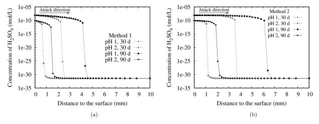
Figure 6.17: The calculated penetration of  $H_2SO_4$  with different pH: (a) Method 1; (b) Method 2.
