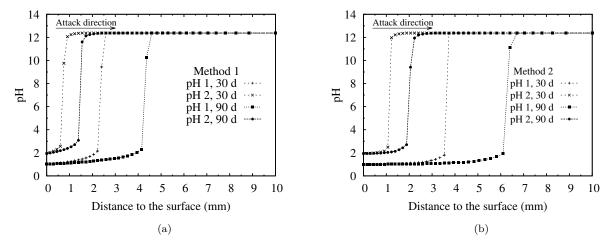
Figure 6.18: The evolution of pH with different pH: (a) Method 1; (b) Method 2.
