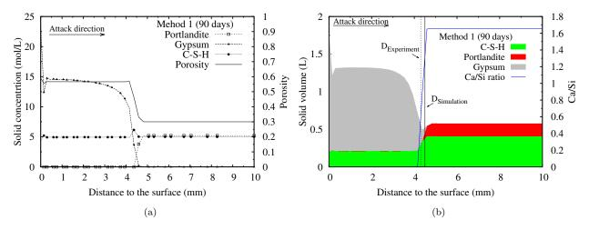
Figure 6.5: After 90 days of immersion: (a) Solid concentration and porosity; (b) Solid volume and Ca/Si ratio of C-S-H .  $D_{Simulation}$  and  $D_{Experiment}$  represent the degradation depth of the sample in simulation and experiment individually. (Method 1, pH = 1)
