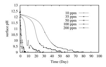
Figure 7.24: The lag time of surface neutralization process with different H<sub>2</sub>S level.
