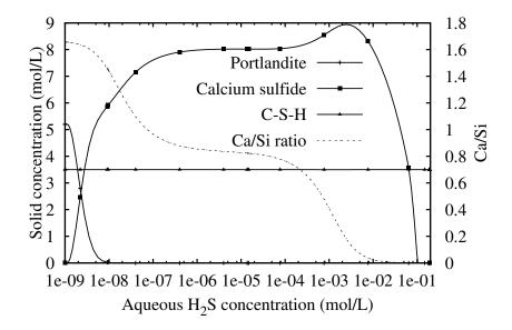
Figure 3.5: Evolution of the solid composition vs. H<sub>2</sub>S concentration in REV of cement paste
