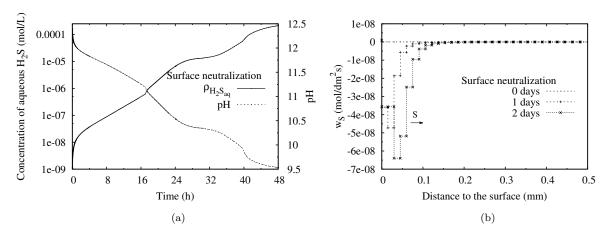
Figure 7.5: The calculated absorption of  $H_2S$  profiles from 0 days to 2 days: (a) Aqueous  $H_2S$  concentration and pH evolution at surface; (b) Diffusion of sulfur. ( $H_2S$  level = 200 ppm)
