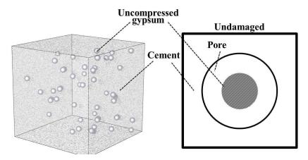
Figure 4.4: Schematics of the microstructure of cementitous materials with uncompressed gypsum inclusion
