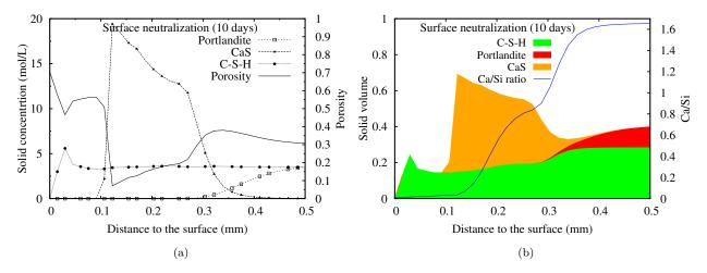
Figure 7.9: After 10 days of exposure: (a) Solid concentration and porosity; (b) Solid volume and Ca/Si ratio of C-S-H. (H<sub>2</sub>S level = 200 ppm)
