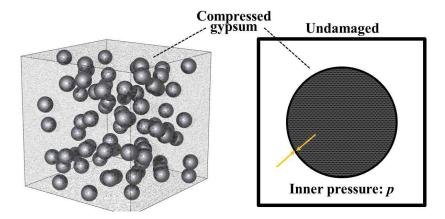
Figure 4.5: Schematics of the microstructure of cementitous materials with compressed gypsum inclusion
