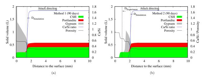
Figure 6.21: The evolution of solid volume, Ca/Si ration of C-S-H and porosity after 90 days immersion : (a) Method 1; (b) Method 2. (pH = 2)
