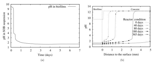
Figure 7.19: The calculated pH evolution profiles (a) pH evolution in biofilms; (b) pH change in biofilms and mortar. (H<sub>2</sub>S level = 400 ppm)
