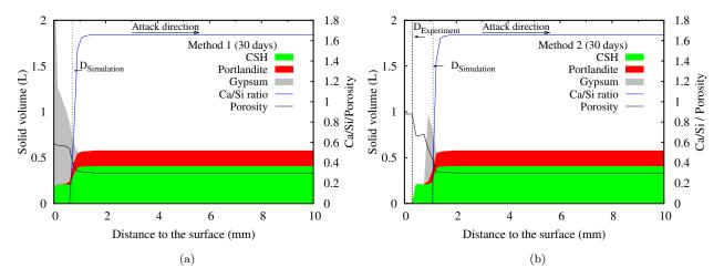
Figure 6.20: The evolution of solid volume, Ca/Si ration of C-S-H and porosity after 30 days immersion : (a) Method 1; (b) Method 2. (pH = 2)
