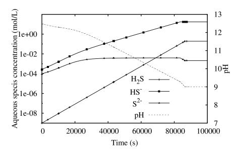
Figure 3.4: Concentration of H<sub>2</sub>S species and pH vs. time in REV of cement paste
