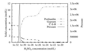
Figure 4.11: Evolution of inner pressure vs. content of CH and  $C\bar{S}H2$  in REV of cement paste
