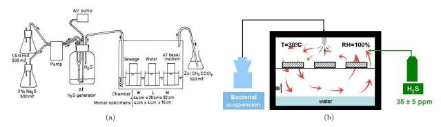
Figure 7.2: Experiment setup of biodeterioration by simulation reactors: (a) (Mori et al., 1992); (b) (Herisson, 2012).
