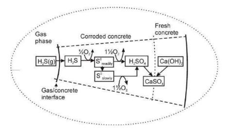
Figure 2.1: Schematic outline of the H<sub>2</sub>S production process. (Jensen et al., 2008)
