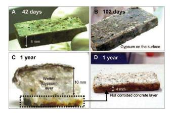
Figure 4.12: Concrete coupons exposed to the sewer atmosphere [H<sub>2</sub>S, 30 ppm] for 42 days (A), 102 days (B), and 1 year (C and D), showing the progression of concrete corrosion. (Okabe et al., 2007)
