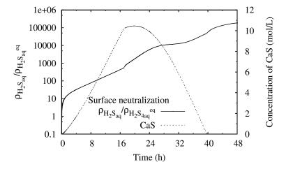
Figure 7.8: The concentration of CaS and aqueous  $H_2S$  at surface from 0 days to 2 days ( $H_2S$  level =200 ppm)
