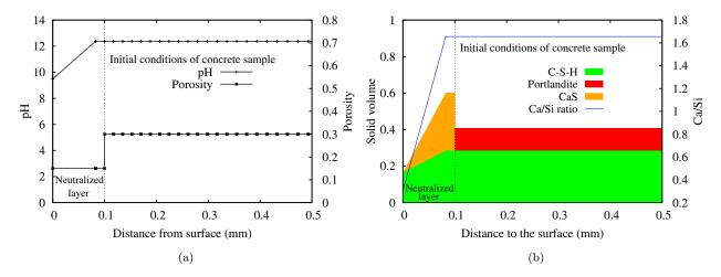
Figure 7.11: Initial concrete sample with neutralized surface: (a) pH and porosity; (b) Solid volume and Ca/Si ratio of C-S-H.
