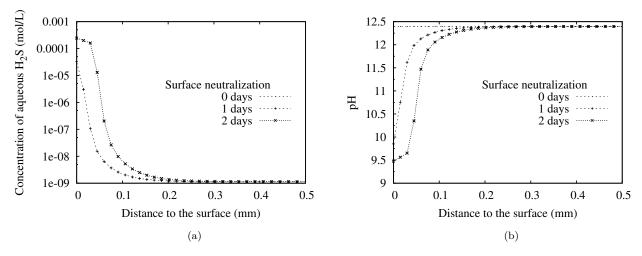
Figure 7.4: The calculated absorption of  $H_2S$  and pH evolution profiles from 0 days to 2 days: (a) Aqueous  $H_2S$  concentration; (b) pH value. ( $H_2S$  level = 200 ppm)
