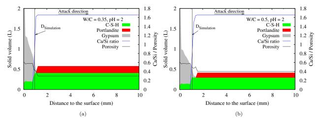
Figure 6.29: Solid compositions, Ca/Si ratio of C-S-H and porosity profiles after 30 days of immersion high  $H_2SO_4$  concentration condition (pH = 2): (a) initial porosity = 0.3; (b) initial porosity = 0.4
