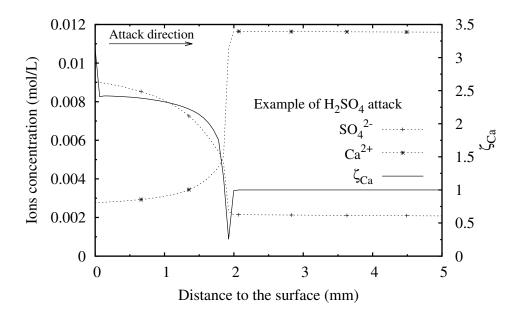
Figure 5.6: Concentration of SO<sub>4</sub><sup>2-</sup> and Ca<sup>2+</sup> and  $\zeta_{\rm Ca}$  after 15 days immersion
