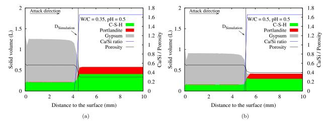
Figure 6.28: Solid compositions, Ca/Si ratio of C-S-H and porosity profiles after 30 days of immersion under high  $H_2SO_4$  concentration condition (pH = 0.5): (a) W/C = 0.35; (b) W/C = 0.5
