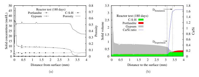
Figure 7.22: After 180 days of test in simulation reactor: (a) Solid concentration and porosity; (b) Solid volume and Ca/Si ratio of C-S-H. (H<sub>2</sub>S level = 400 ppm)
