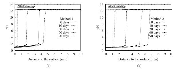
Figure 6.25: The evolution of pH from 10 days to 90 days for the sample with carbonated layer: (a) Method 1; (b) Method 2. (pH = 1)
