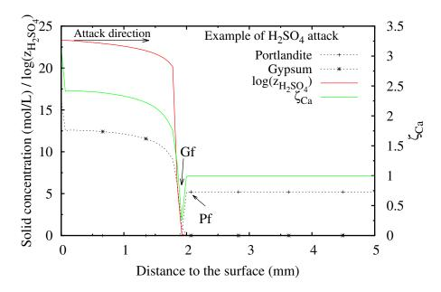
Figure 5.5: CH and CSH2 content,  $\zeta_{\text{Ca}}$  and  $\log(z_{\text{H}_2\text{SO}_4})$  after 15 days immersion
