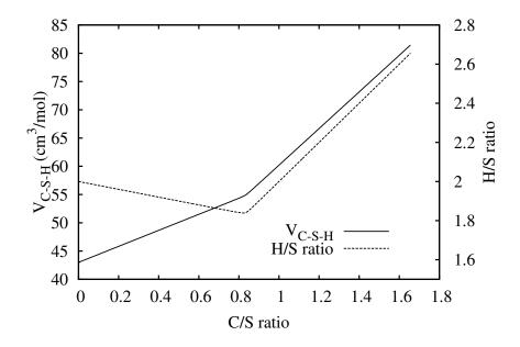
Figure 4.1:  $V_{\text{C-S-H}}$  and  $\text{H}_2\text{O/Si}$  ratio z vs. Ca/Si ratio x.
