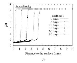
Figure 6.2: The calculated penetration of  $H_2SO_4$  and pH evolution profiles from 0 days to 90 days: (a)  $H_2SO_4$  concentration; (b) pH value. (Method 1, pH = 1)
