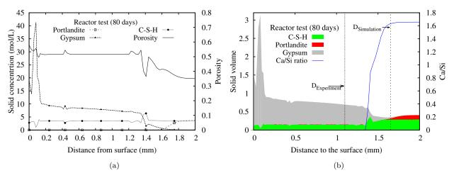
Figure 7.21: After 80 days of test in simulation reactor: (a) Solid concentration and porosity; (b) Solid volume and Ca/Si ratio of C-S-H. ( $H_2S$  level = 400 ppm)
