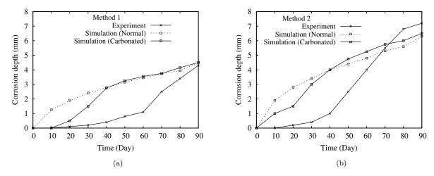
Figure 6.27: The corrosion depth profiles of simulation and experiments from 10 days to 90 days: (a) Method 1; (b) Method 2
