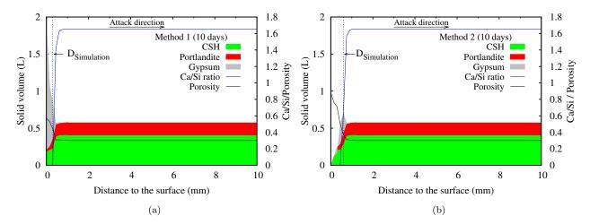
Figure 6.19: The evolution of solid volume, Ca/Si ration of C-S-H and porosity after 10 days immersion : (a) Method 1; (b) Method 2. (pH = 2)
