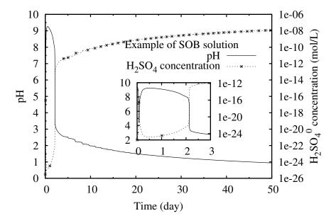
Figure 5.11: pH and H<sub>2</sub>SO<sub>4</sub> concentration in SOB solution containing cement paste
