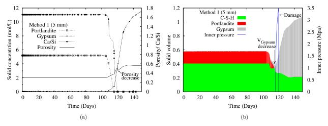
Figure 6.6: At 5 mm depth of sample (a) Solid concentration, Ca/Si ratio of C-S-H and porosity; (b) Solid volume and inner pressure. (Method 1, pH = 1)
