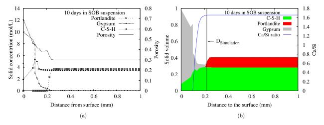
Figure 7.14: After 10 days of immersion in SOB suspension: (a) Solid concentration and porosity; (b) Solid volume and Ca/Si ratio of C-S-H.  $D_{Simulation}$  represents the degradation depth of the sample in simulation
