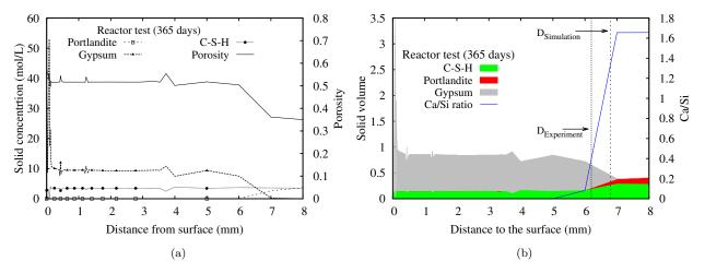
Figure 7.23: After 1 year of test in simulation reactor: (a) Solid concentration and porosity; (b) Solid volume and Ca/Si ratio of C-S-H. (H<sub>2</sub>S level = 400 ppm)
