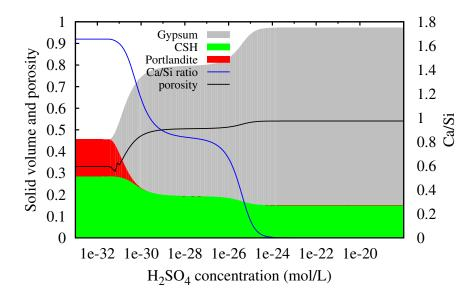
Figure 4.10: Evolution of the solid volume and porosity vs. H<sub>2</sub>SO<sub>4</sub> concentration in REV of cement paste
