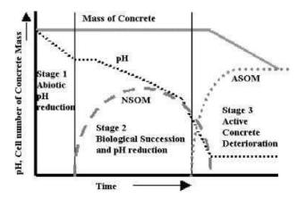
Figure 1.4: Theoretical changes in the biological and physical properties of concrete with time during the deterioration process, (Islander et al., 1991).
