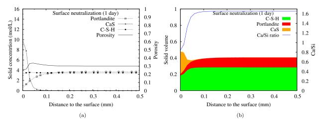
Figure 7.6: After 1 day of exposure: (a) Solid concentration and porosity; (b) Solid volume and Ca/Si ratio of C-S-H. ( $H_2S$  level = 200 ppm)
