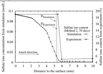
Figure 6.16: The concentration of  $HSO_4^-$  and  $SO_4^{2-}$  in the sample after 70 days immersion. (Method 2, pH = 1)
