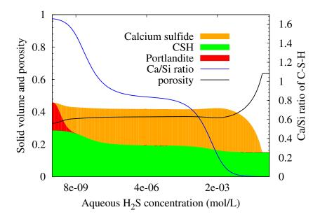
Figure 4.9: Evolution of the solid volume and porosity vs. H<sub>2</sub>S concentration in REV of cement paste
