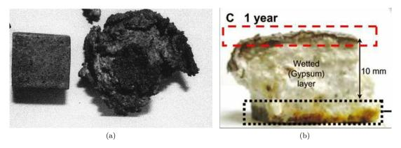
Figure 4.2: (a) OPC Mortar after 350 Days of biogenic sulfuric acid corrosion in simulation chamber. Samples on left side is reference sample, whereas on right side sample exposed to corrosion condition. (Ehrich et al., 1999); (b) The appearance of concrete coupons exposed to the sewer atmosphere for 1 year. (Okabe et al., 2007)
