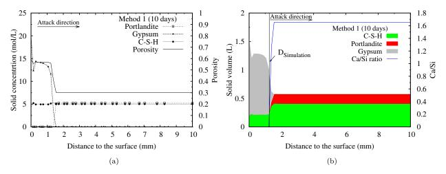
Figure 6.3: After 10 days of immersion: (a) Solid concentration and porosity; (b) Solid volume and Ca/Si ratio of C-S-H .  $D_{Simulation}$  and  $D_{Experiment}$  represent the degradation depth of the sample in simulation and experiment individually. (Method 1, pH = 1)
