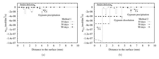
Figure 6.14: The calculated diffusion of calcium during immersion: (a) Method 1; (b) Method 2. (pH = 1)
