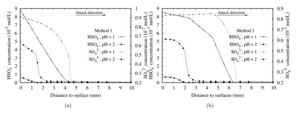
Figure 6.22: The concentration of  $HSO_4^-$  and  $SO_4^{2-}$  after 90 days immersion with different pH: (a) Method 1; (b) Method 2.
