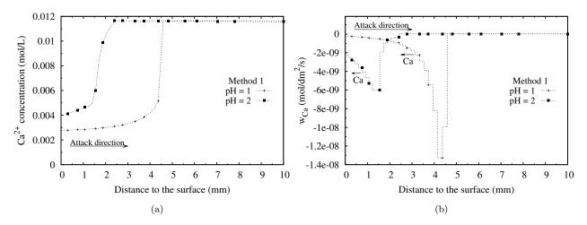
Figure 6.24: After 90 days immersion: (a) The concentration of Ca<sup>2+</sup>1; (b) Flux of calcium (Method 1)
