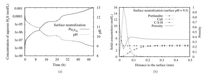
Figure 7.17: When surface pH decreases to 9.5: (a) Aqueous  $H_2S$  concentration and pH evolution at surface; (b) Solid concentration and porosity of mortar sample. ( $H_2S$  level = 400 ppm)
