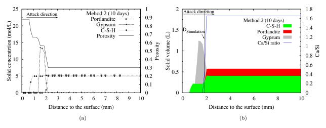
Figure 6.10: After 10 days of immersion: (a) Solid concentration and porosity; (b) Solid volume and Ca/Si ratio of C-S-H .  $D_{Simulation}$  and  $D_{Experiment}$  represent the degradation depth of the sample in simulation and experiment individually. (Method 2, pH = 1)
