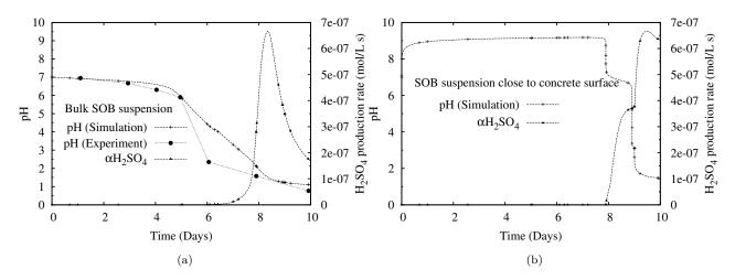
Figure 7.13: The pH evolution and production rate of  $H_2SO_4$  from 0 to 10 days: (a) bulk SOB suspension; (b) SOB closed to concrete surface.
