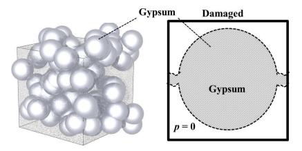
Figure 4.8: Schematics of the microstructure of damaged cementitous materials
