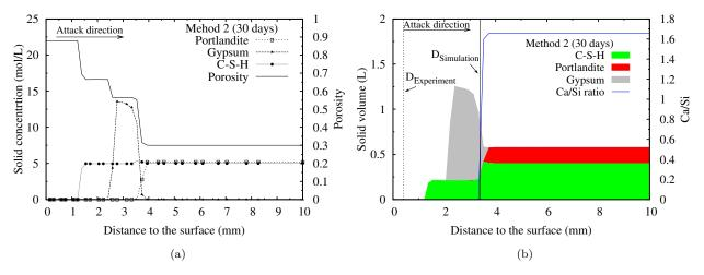
Figure 6.11: After 30 days of immersion: (a) Solid concentration and porosity; (b) Solid volume and Ca/Si ratio of C-S-H .  $D_{Simulation}$  and  $D_{Experiment}$  represent the degradation depth of the sample in simulation and experiment individually. (Method 2, pH = 1)
