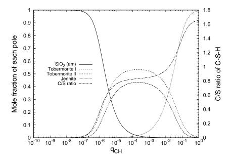
Figure A.3: Mole fraction of different poles and Ca/Si evolution  $vs. q_{CH}$ .
