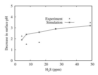
Figure 2.4: Decrease in surface pH ( $pH_{\text{(initial)}} - pH_{\text{(exposed)}}$ ) after 1 year.
