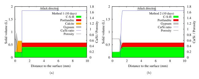
Figure 6.26: The evolution of solid volume, Ca/Si ration of C-S-H and porosity of samples with carbonated layer after 10 days immersion: (a) Method 1; (b) Method 2. (pH = 1)
