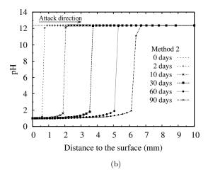
Figure 6.9: The calculated penetration of  $H_2SO_4$  and pH evolution profiles from 0 days to 90 days: (a)  $H_2SO_4$  concentration; (b) pH value. (Method 2, pH = 1)
