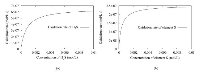
Figure 2.9: Oxidation rate: (a)  $H_2S$ ; (b) element S.
