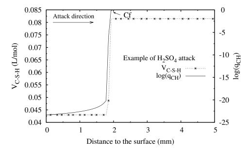
Figure 5.9:  $V_{\text{C-S-H}}$  of C-S-H and  $\log(q_{\text{CH}})$  after 15 days immersion
