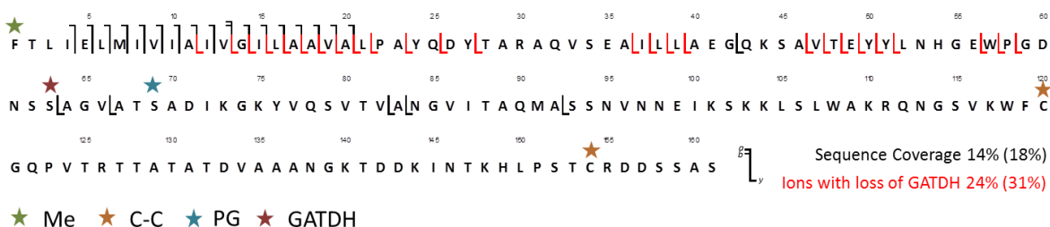
Figure 114 - Fragmentation map from 12 eV CAD FT-ICR MS/MS of the 17+ charge state of PilE-8013. Ions exhibiting loss of GATDH are highlighted in red
