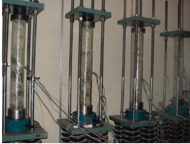
Figure 2.3: Photo of uniaxial compressive creep testing machine [Lee et al., 2006].
